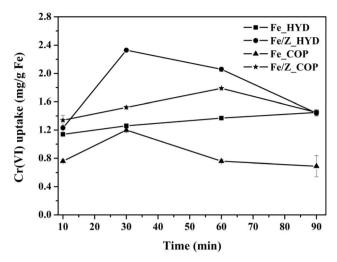
Fig. 8 Effect of contact time to the adsorption capacity of all samples (condition:  $Cr(v_i)$  initial concentration = 1 ppm, pH 2 for Fe/Z\_HYD, pH 3 for F\_HYD, Fe\_COP, Fe/Z\_COP and temperature 30 °C).
