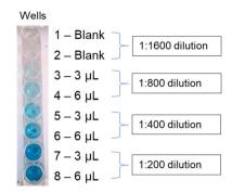
Fig. 7 Testing of spiked cow milk samples for hydrogen peroxide using immobilized Strep-HRP kit.
