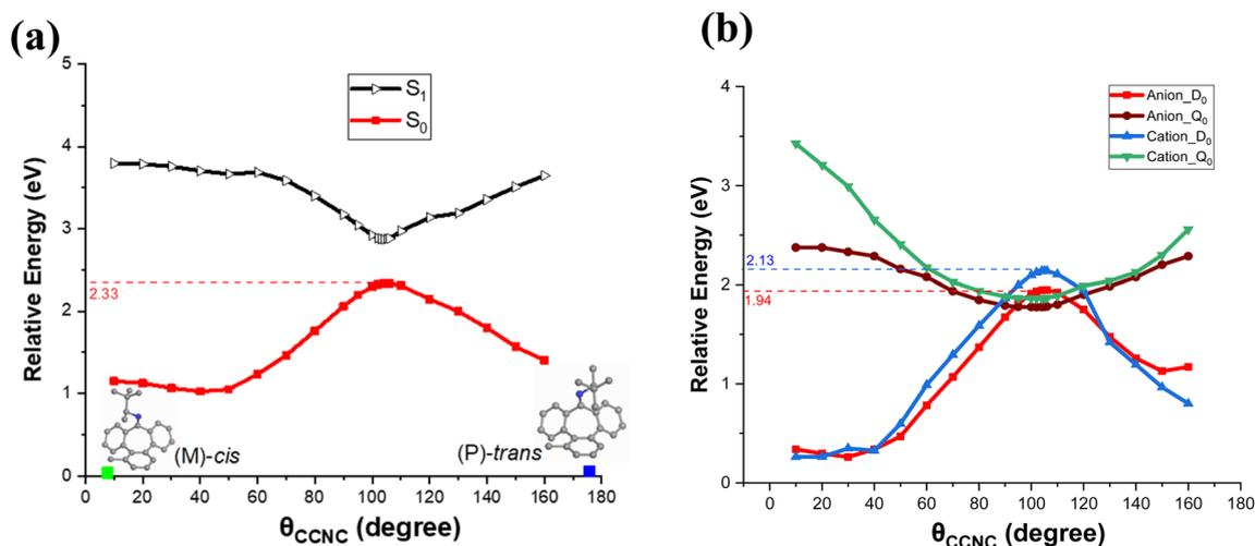
Fig. 3 Relative energy profiles of neutral and charged molecules. (a) Neutral molecule in the singlet excited state ( $S_1$ ) and ground state ( $S_0$ ) for the photoisomerization process. The optimized molecular structures are displayed in the inset without hydrogens for clarity. (b) Charged molecule in doublet spin state ( $D_0$ ) and quartet spin state ( $Q_0$ ).
