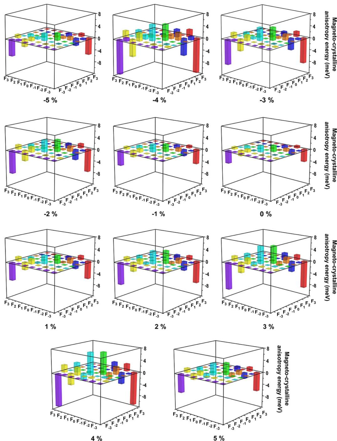
Fig. 8 Resolved magneto-crystalline anisotropy energies (MAE) of Ce-f orbitals for CeFCl monolayer under biaxial strain from  $-5\%$  to  $5\%$ ,  $F_{-3}$ ,  $F_{-2}$ ,  $F_{-1}$ ,  $F_0$ ,  $F_1$ ,  $F_2$  and  $F_3$  orbitals represent  $f_{y(3x^2-y^2)}$ ,  $f_{xyz}$ ,  $f_{yz^2}$ ,  $f_{z^3}$ ,  $f_{xz^2}$ ,  $f_{z(x^2-y^2)}$  and  $f_{x(x^2-3y^2)}$  orbitals, respectively.
