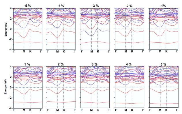
Spin-resolved band structure for CeFCl monolayer under biaxial strain from -5% to 5%
