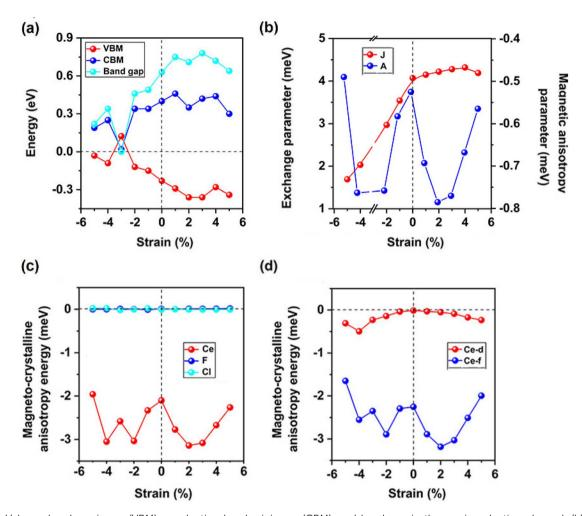
Fig. 6 (a) Valence band maximum (VBM), conduction band minimum (CBM), and band gap in the semiconducting channel, (b) exchange parameter J and magnetic anisotropy parameter A, the magneto-crystalline anisotropy energies (MAE) of (c) Ce, F, and Cl ions, and projected on (d) Ce-d/f orbitals for CeFCl monolayer under biaxial strain from -5% to 5%.
