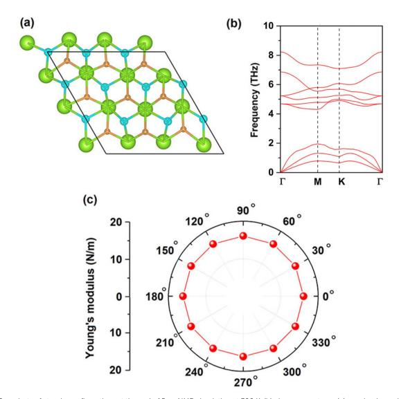
Fig. 4 (a) Snapshots of atomic configurations at the end of 5 ps AIMD simulation at 300 K, (b) phonon spectrum, (c) angular dependence of the Young's modulus for CeFCI monolayer.
