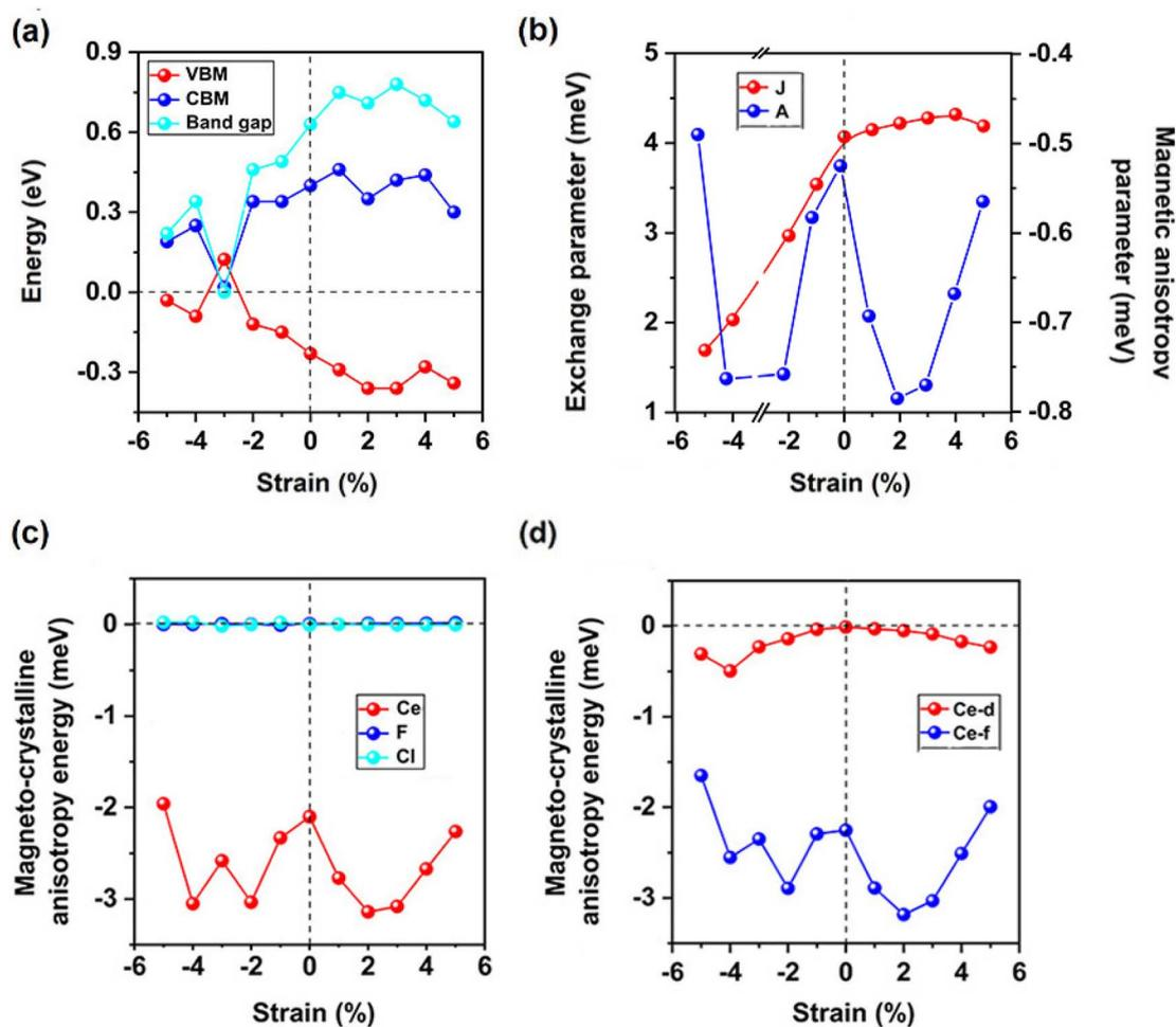
Fig. 6 (a) Valence band maximum (VBM), conduction band minimum (CBM), and band gap in the semiconducting channel, (b) exchange parameter  $J$  and magnetic anisotropy parameter  $A$ , the magneto-crystalline anisotropy energies (MAE) of (c) Ce, F, and Cl ions, and projected on (d) Ce-d/f orbitals for CeFCI monolayer under biaxial strain from  $-5\%$  to  $5\%$ .
