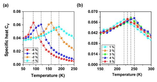
Fig. 7 (a) and (b) the simulated averaged specific heat with respect to temperature for CeFCl monolayer under biaxial strain from -5% to 5%.
