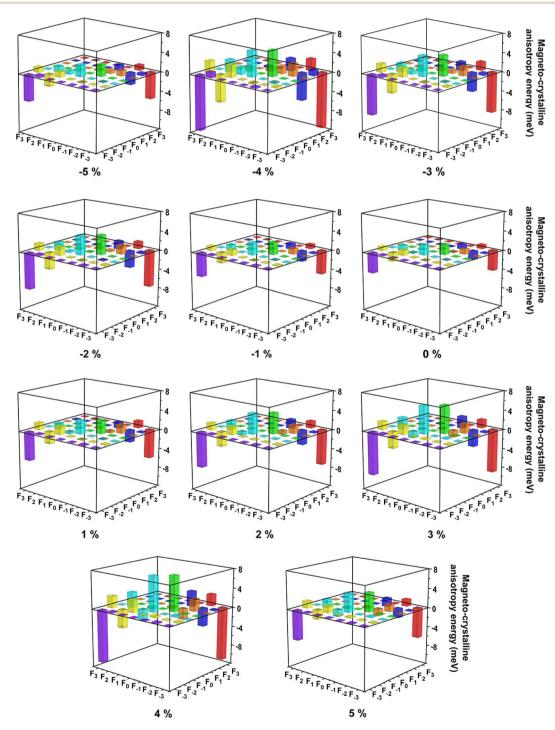
Fig. 8 Resolved magneto-crystalline anisotropy energies (MAE) of Ce-f orbitals for CeFCI monolayer under biaxial strain from -5% to 5%, F<sub>-3</sub>,  $F_{-2}, \, F_{-1}, \, F_0, \, F_1, \, F_2 \, \text{ and } F_3 \, \text{ orbitals represent } f_{y(3x^2-y^2)}, \, f_{xyz}, \, f_{yz^2}, \, f_{z^3}, \, f_{xz^2}, \, f_{z(x^2-y^2)} \, \text{ and } f_{x(x^2-3y^2)} \, \text{ orbitals, respectively.}$
