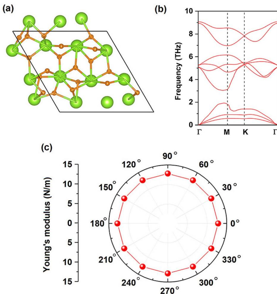
Fig. 2 (a) Snapshots of atomic configurations at the end of 5 ps AIMD simulation at 300 K, (b) phonon spectrum, (c) angular dependence of the Young's modulus for CeF<sub>2</sub> monolayer.
