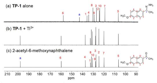
Fig. 3 Partial  $^{13}$ C NMR spectra of (a) TP-1, (b) TP-1 + Tl $^{3+}$ , and (c) 2-acetyl-6-methoxynaphthalene in DMSO- $d_6$ . [TP-1] = [2-acetyl-6-methoxynaphthalene] = 5.0 mM. For (b), the spectrum (TP-1 + Tl $^{3+}$ ) was obtained using a purified product of a mixture of TP-1 (5.0 mM) and Tl(NO $_3$ )<sub>3</sub> (10.0 mM) in acetate buffer (pH 4.8) containing 1% (v/v) DMF.
