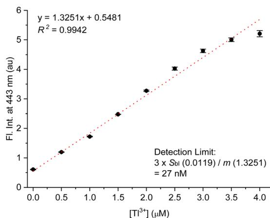
Fig. 5 Concentration-dependent  $Tl^{3+}$  signaling of TP-1 in artificial urine. [TP-1] = 5.0  $\mu M$ ,  $[Tl^{3+}]$  = 0–4  $\mu M$ , [buffer] = 10 mM in a pH 4.8 acetate buffered artificial urine solution containing 1% (v/v) DMF.  $\lambda_{ex}$  = 309 nm.
