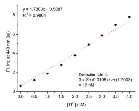
Fig. 4 Calibration curve for fluorescence titration of TP-1 with Tl<sup>3+</sup>  $[TP-1] = 5.0 \mu M$ ,  $[Tl^{3+}] = 0-4.0 \mu M$ , in a pH 4.8 acetate buffer solution (10 mM) containing 1% (v/v) DMF.  $\lambda_{ex} = 309$  nm.
