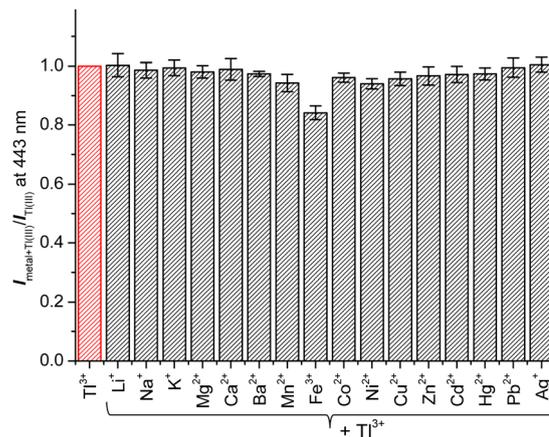
Fig. 2 Changes in fluorescence intensity ratio ( $I_{\text{metal+Tl(m)}}/I_{\text{Tl(m)}}$ ) of **TP-1** at 443 nm in the presence of coexisting metal ions. [**TP-1**] = 5.0  $\mu$ M, [Tl<sup>3+</sup>] = [M<sup>n+</sup>] = 50  $\mu$ M, in a pH 4.8 acetate buffer solution (10 mM) containing 1% (v/v) DMF.  $\lambda_{\text{ex}}$  = 309 nm.
