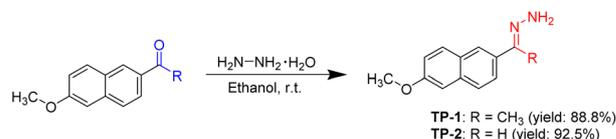
Scheme 1 Preparation of Tl<sup>3+</sup> signaling probes **TP-1** and **TP-2**.
