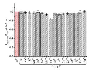
Fig. 2 Changes in fluorescence intensity ratio ( $I_{metal+TI(iii)}/I_{TI(iii)}$ ) of TP-1 at 443 nm in the presence of coexisting metal ions. [TP-1] = 5.0  $\mu$ M, [TI<sup>3+</sup>] = [M<sup>n+</sup>] = 50  $\mu$ M, in a pH 4.8 acetate buffer solution (10 mM) containing 1% (v/v) DMF.  $\lambda_{ex}$  = 309 nm.
