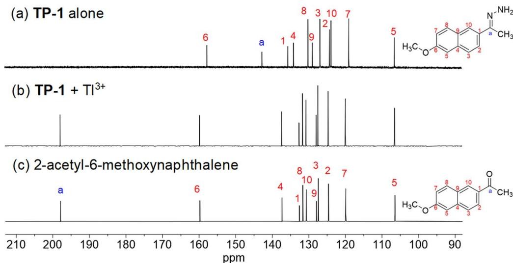
Fig. 3 Partial  $^{13}C$  NMR spectra of (a) TP-1, (b) TP-1 +  $Tl^{3+}$ , and (c) 2-acetyl-6-methoxynaphthalene in  $DMSO-d_6$ . [TP-1] = [2-acetyl-6-methoxynaphthalene] = 5.0 mM. For (b), the spectrum (TP-1 +  $Tl^{3+}$ ) was obtained using a purified product of a mixture of TP-1 (5.0 mM) and  $Tl(NO_3)_3$  (10.0 mM) in acetate buffer (pH 4.8) containing 1% (v/v) DMF.
