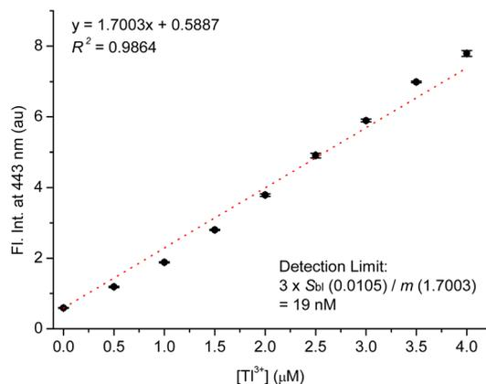
Fig. 4 Calibration curve for fluorescence titration of TP-1 with  $Tl^{3+}$ . [TP-1] = 5.0  $\mu M$ ,  $[Tl^{3+}]$  = 0–4.0  $\mu M$ , in a pH 4.8 acetate buffer solution (10 mM) containing 1% (v/v) DMF.  $\lambda_{ex}$  = 309 nm.
