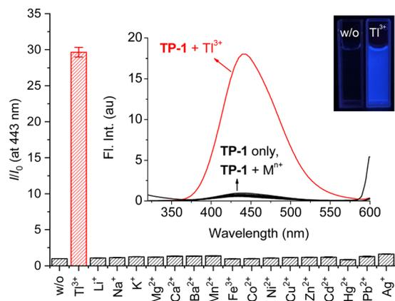
Fig. 1 Changes in fluorescence intensity enhancement ( $I/I_0$ ) at 443 nm of **TP-1** in the presence of common metal ions. Inset: fluorescence spectra and fluorescence image of **TP-1**. [**TP-1**] = 5.0  $\mu$ M, [Tl<sup>3+</sup>] = [M<sup>n+</sup>] = 50  $\mu$ M, in a pH 4.8 acetate buffer solution (10 mM) containing 1% (v/v) DMF.  $\lambda_{\text{ex}}$  = 309 nm.
