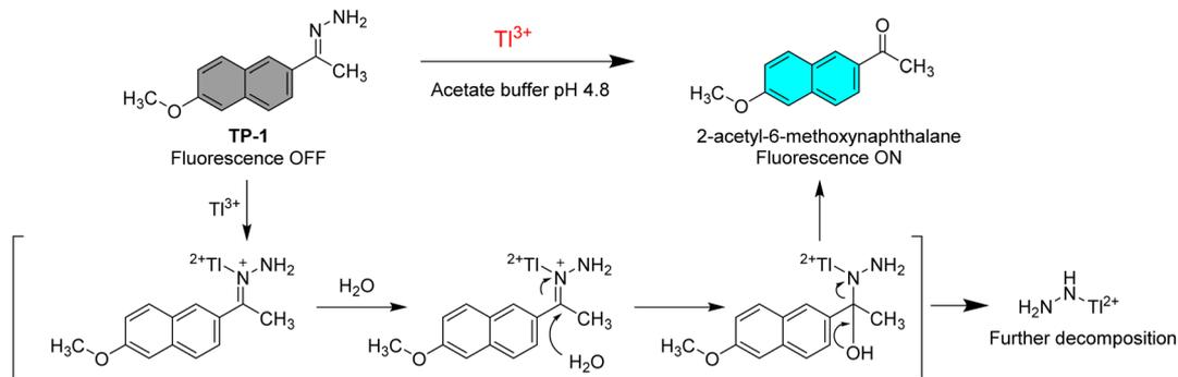
Scheme 2 Suggested  $Tl^{3+}$  sensing mechanism of TP-1.
