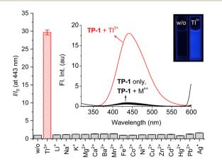
Fig. 1 Changes in fluorescence intensity enhancement (///<sub>0</sub>) at 443 nm of TP-1 in the presence of common metal ions. Inset: fluorescence spectra and fluorescence image of TP-1. [TP-1] = 5.0  $\mu$ M, [Tl<sup>3+</sup>] = [M<sup>n+</sup>] = 50  $\mu$ M, in a pH 4.8 acetate buffer solution (10 mM) containing 1% (v/v) DMF.  $\lambda_{ex}$  = 309 nm.
