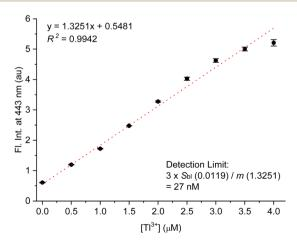
Fig. 5 Concentration-dependent Tl<sup>3+</sup> signaling of TP-1 in artificial urine. [TP-1] = 5.0  $\mu$ M, [Tl<sup>3+</sup>] = 0-4  $\mu$ M, [buffer] = 10 mM in a pH 4.8 acetate buffered artificial urine solution containing 1% (v/v) DMF.  $\lambda_{ex} =$ 309 nm.
