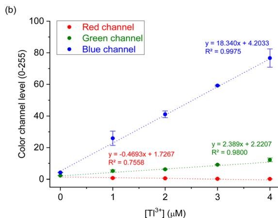
Fig. 6 (a) Fluorescence and its color filtered (RGB) images of TP-1 as increased of  $[Tl^{3+}]$  in urine solution. (b) Calibration curve of the color channel level versus  $[Tl^{3+}]$  concentration. [TP-1] = 5.0  $\mu M$ ,  $[Tl^{3+}]$  = 0–4.0  $\mu M$ , [buffer] = 10 mM in artificial urine solution containing 1% (v/v) DMF.
