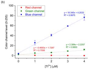
Fig. 6 (a) Fluorescence and its color filtered (RGB) images of TP-1 as increased of [Tl<sup>3+</sup>] in urine solution. (b) Calibration curve of the color channel level versus [ $Tl^{3+}$ ] concentration. [TP-1] = 5.0  $\mu$ M, [ $Tl^{3+}$ ] = 0-4.0  $\mu$ M, [buffer] = 10 mM in artificial urine solution containing 1% (v/v) DMF.
