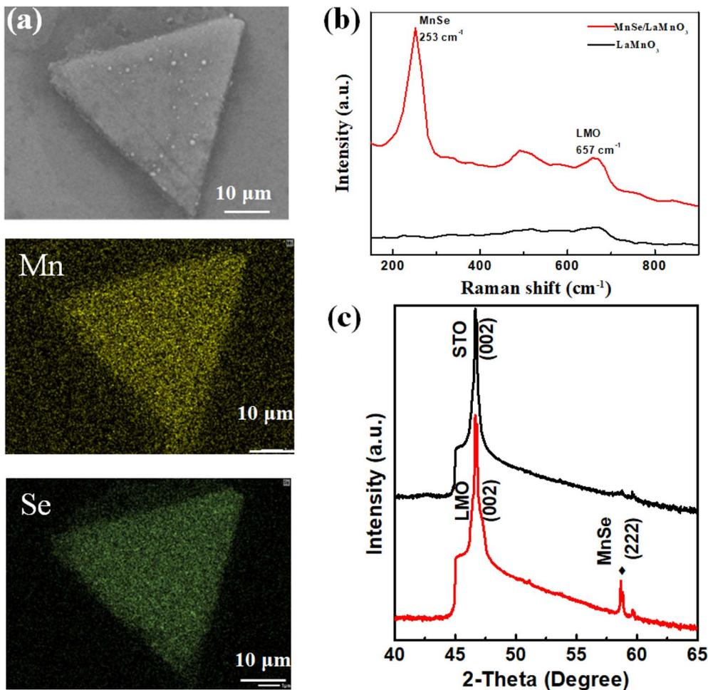
Fig. 1 (a) SEM image of MnSe/LMO heterostructure. Mn and Se elemental images of MnSe/LMO heterostructure. (b) Raman spectra of MnSe/LMO heterostructure and the reference single LMO film. (c) XRD patterns of the obtained MnSe/LMO heterostructure and the reference single LMO film. The  $\blacklozenge$  symbol is labeled as MnSe peak.
