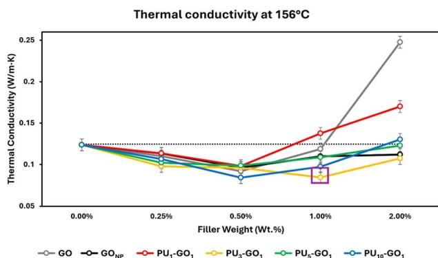
Fig. 3 Thermal conductivity of PU foams with varying weight percents of each filler. It is important to note that lower thermal conductivity indicates a greater capacity for thermal insulation. A purple box is drawn around PU<sub>3</sub>-GO<sub>1</sub> 1.0%, the only sample where the lowest thermal conductivity did not occur at 0.5% filler content.
