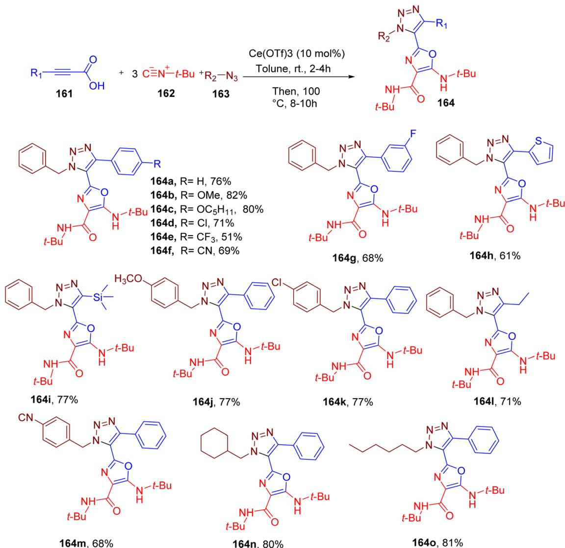
Fig. 41 MCR for the simultaneous synthesis of triazole-oxazole-based derivatives.
