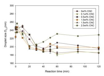
Fig. 5 Droplet size of each sample during the reaction as a function of CNC content.
