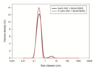
Fig. 2 Variation in initial droplet size distribution with or without 0.1wt% CNC in water phase (30 mM SDSO).
