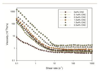
Fig. 6 Variation in viscosity *versus* shear rate as a function of CNC content.
