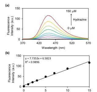
Fig. 4 (a) Fluorescence spectra and (b) Plot of fluorescence intensity at 447 nm of OB-MU3 (10  $\mu$ M) with different equivalents of hydrazine (0, 1, 2, 3, 5, 7, 10, and 15 eq.) in 50 mM HEPES buffer (1% acetonitrile, pH 7.4) at 25 °C, 30 min after addition of hydrazine ( $\lambda_{ex}$ : 323 nm).
