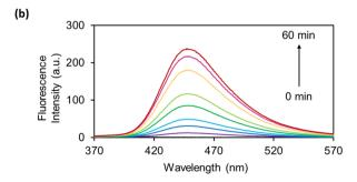
Fig. 3 Fluorescence spectra of (a) OB-MU2 (10 μM) and (b) OB-MU3 (10  $\mu$ M) in the presence of hydrazine (200  $\mu$ M) in 50 mM HEPES buffer (1% acetonitrile, pH 7.4) at 25 °C for 0, 1, 3, 5, 10, 15, 30, 45, and 60 min  $(\lambda_{ex}: 323 \text{ nm}, \lambda_{em}: 370-570 \text{ nm}).$
