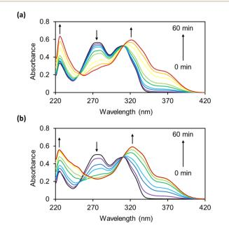
Fig. 1 UV-vis spectra of (a) OB-MU2 (50  $\mu$ M) and (b) OB-MU3 (50  $\mu$ M) in the presence of hydrazine (1 mM) in 50 mM HEPES buffer (1% acetonitrile, pH 7.4) at 25 °C for 0, 1, 3, 5, 10, 15, 30, 45, and 60 min.
