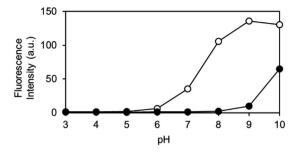
Fig. 6 Fluorescent intensity of OB-MU3 (10  $\mu$ M) under a variety of pH conditions (1% acetonitrile) after 30 min incubation with (200  $\mu$ M, open circles) or without (0  $\mu$ M, closed circles) hydrazine ( $\lambda_{ex}$ : 323 nm,  $\lambda_{em}$ : 447 nm)
