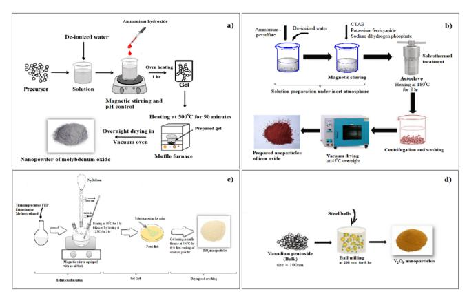
Fig. 1 Schematics of the synthesis of metal oxide nanoparticles: (a) molybdenum trioxide ( $MoO_3$ ) nanoparticles. (b) Ferric oxide ( $Fe_2O_3$ ) nanoparticles. (c) Titanium dioxide ( $TiO_2$ ) nanoparticles. (d) Vanadium pentoxide ( $V_2O_5$ ) nanoparticles.
