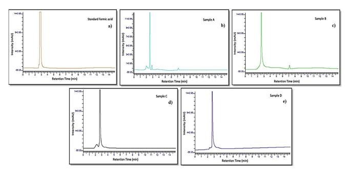
Fig. 6 HPLC chromatographs of (a) standard formic acid (200 ppm), (b) sample A (200 ppm), (c) sample B (200 ppm), (d) sample C (200 ppm) and (e) sample D (200 ppm).
