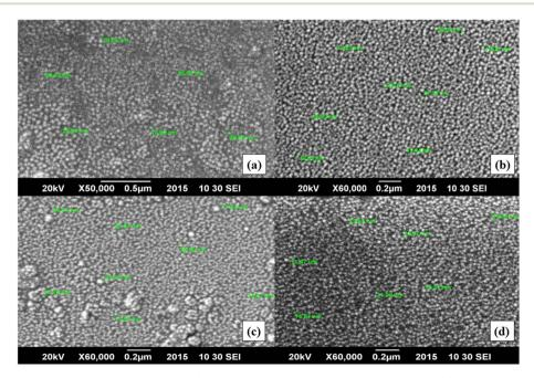
Fig. 3 SEM micrographs of the prepared nanoparticles: (a) molybdenum trioxide (MoO<sub>3</sub>) nanoparticles. (b) Iron oxide (Fe<sub>2</sub>O<sub>3</sub>) nanoparticles. (c) Titanium oxide (TiO<sub>2</sub>) nanoparticles. (d) Vanadium pentoxide ( $V_2O_5$ ) nanoparticles.
