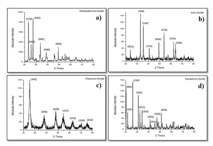
Fig. 5 XRD patterns of (a) molybdenum trioxide ( $MoO_3$ ) nanoparticles, (b) iron oxide ( $Fe_2O_3$ ) nanoparticles, (c) titanium oxide ( $TiO_2$ ) nanoparticles and (d) vanadium pentoxide ( $V_2O_5$ ) nanoparticles.
