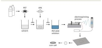
Fig. 1 Flow of recycled PET-based battery separator synthesis from waste plastic bottles via the electrospinning process.
