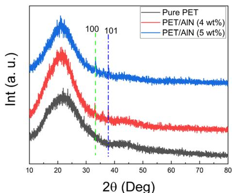
Fig. 3 XRD spectrum of PET/AlN 4 wt% and PET/AlN 5 wt% vs. pure PET.
