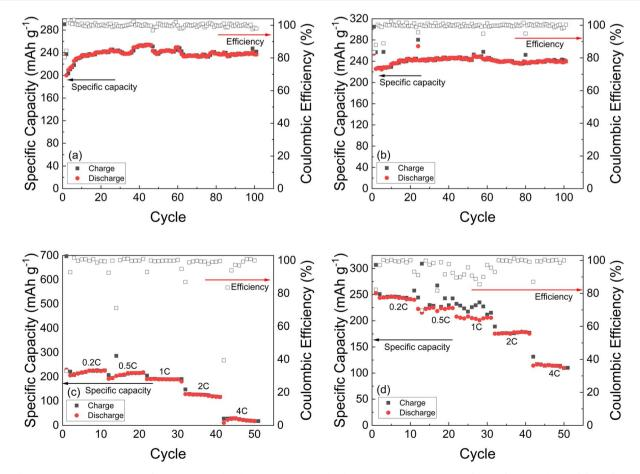
Fig. 9 Cycling performance of PET/AIN-based CR2032 coin batteries at 0.5C with different separators: (a) PET/AIN 4 wt% and (b) PET/AIN 5 wt%, and under different C-rate (0.2C, 0.5C, 1C, 2C, 4C) (c) PET/AIN 4 wt%, and (d) PET/AIN 5 wt%.
