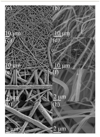
Fig. 10 SEM images of (a) spent vs. (b) fresh PET/AIN 4 wt% separators and (c) spent vs. (d) fresh PET/AIN 5 wt% separators through galvanostatic performance analysis vs. fresh (scale bar: 10 μm), and corresponding magnified images (PET/AIN 4 wt%: (e) spent vs. fresh (f); PET/ AlN 5 wt%: (g) spent vs. fresh (h)) (scale bar: 2 μm).
