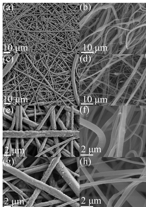
Fig. 10 SEM images of (a) spent vs. (b) fresh PET/AlN 4 wt% separators and (c) spent vs. (d) fresh PET/AlN 5 wt% separators through galvanostatic performance analysis vs. fresh (scale bar: 10 μm), and corresponding magnified images (PET/AlN 4 wt%: (e) spent vs. fresh (f); PET/AlN 5 wt%: (g) spent vs. fresh (h)) (scale bar: 2 μm).
