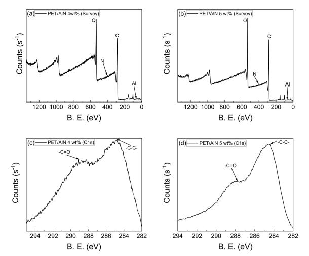
Fig. 5 Survey XPS of (a) PET/AlN 4 wt% and (b) PET/AlN 5 wt%. HR-XPS of C 1s of (c) PET/AlN 4 wt% and (d) PET/AlN 5 wt%.
