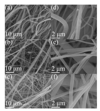
Fig. 2 SEM image of (a) PET/AlN 4 wt%, (b) PET/AlN 5 wt%, and (c) pure PET; corresponding magnified images ((d) PET/AlN 4 wt%, (e) PET/AlN 5 wt%, and (f) pure PET) (scale bar: (a-c) 10  $\mu$ m, (d-f) 2  $\mu$ m).
