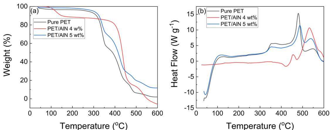
Fig. 7 (a) TGA and (b) DSC spectra of PET/AlN 4 wt%, PET/AlN 5 wt%, and pure PET.
