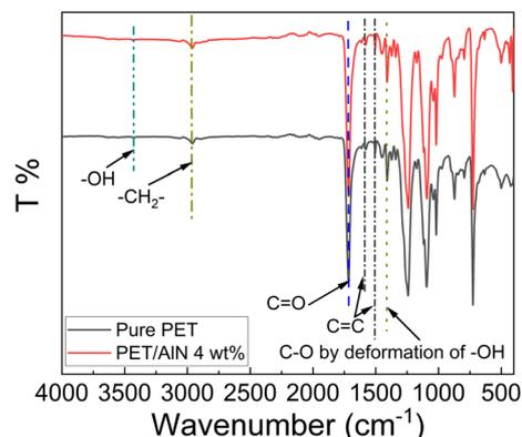
Fig. 4 FTIR spectrum of PET/AlN (4 wt%) vs. pure PET.
