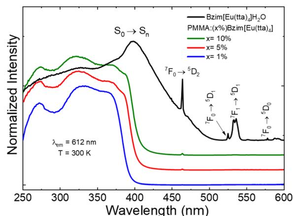
Fig. 5 Excitation spectra of the solid state Bzim[Eu(tta)<sub>4</sub>]·H<sub>2</sub>O complexes and the corresponding PMMA:(x%)Bzim[Eu(tta)<sub>4</sub>] doped films, for which x = 1, 5 and 10% (w/w). All excitation spectra were recorded under room temperature in the 250–600 nm range, monitoring the emission at the hypersensitive <sup>5</sup>D<sub>0</sub> → <sup>7</sup>F<sub>2</sub> transition (λ<sub>em</sub> = 612 nm) of the Eu<sup>3+</sup> ion.
