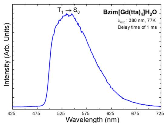
Fig. 4 Phosphorescence spectrum of the solid-state Bzim[Gd(tta)<sub>4</sub>]·H<sub>2</sub>O complex recorded at 77 K from 425 to 725 nm under excitation at 380 nm with 1.0 ms of delay.
