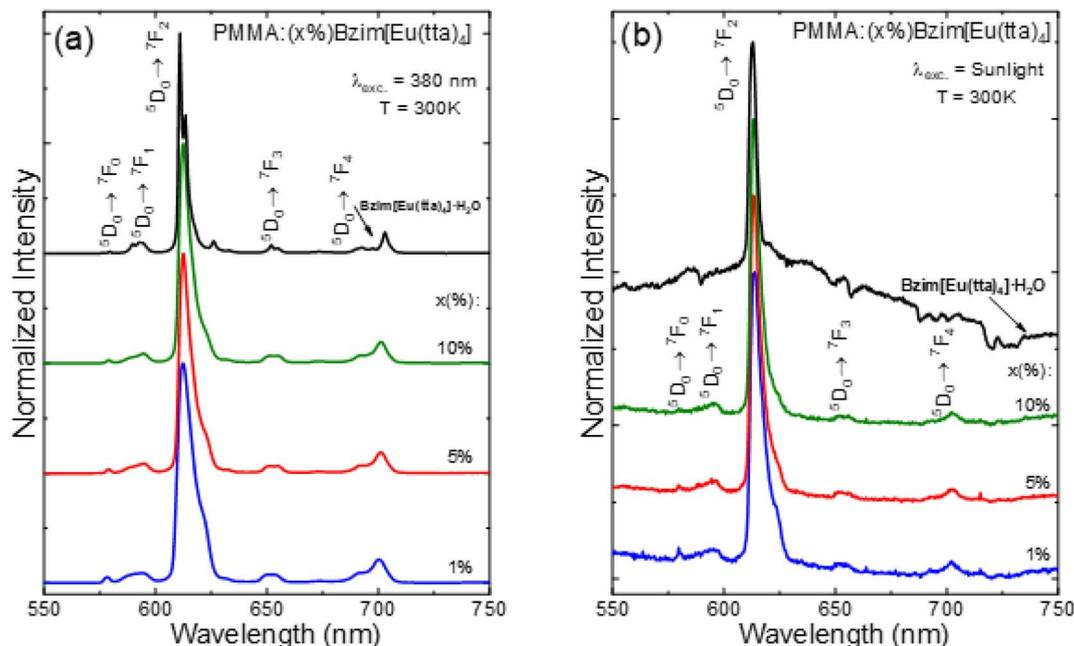
Fig. 6 Emission spectra of the Bzim[Eu(tta)<sub>4</sub>]·H<sub>2</sub>O complex (black line) and the doped PMMA:(x%)Bzim[Eu(tta)<sub>4</sub>] polymers, where x = 1% (blue line), 5% (red line) and 10% (green line) with excitation at 380 nm (a) and under sunlight exposure (b). All spectra were recorded at room temperature in the range of 550 to 750 nm.
