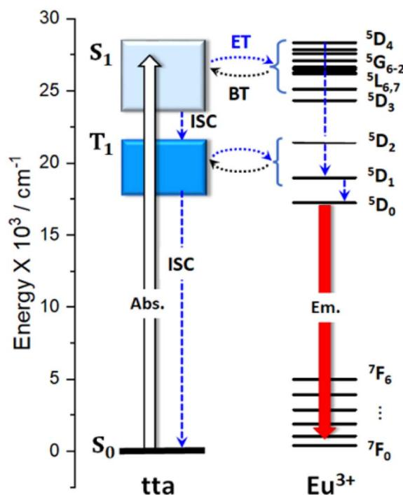
Fig. 7 Partial energy level diagram of the  $\text{Bzim}[\text{Eu}(\text{tta})_4] \cdot \text{H}_2\text{O}$  complex. The emission arises from the  ${}^5D_0$  emitting level.  $S_0$  and  $S_1$  are the ligand ground and lowest singlet excited states, respectively.  $T_1$  is the lowest triplet ligand level, Abs. is the initial absorption, ISC is the intersystem crossing, where Em. is the emission. ET and BT are the forward and backward energy transfer rates, respectively.
