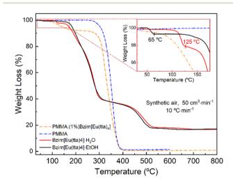
Fig. 3 Thermogravimetric curves of the Bzim[Eu(tta)<sub>4</sub>]·H<sub>2</sub>O and Bzim [Eu(tta)4] · EtOH complexes (solid red and black lines), PMMA:(1%)Bzim [Eu(tta)<sub>4</sub>]-doped film (dashed orange line), and undoped PMMA polymer (dashed blue line). All curves were obtained under a dynamic synthetic air atmosphere of 50 cm $^3$  min $^{-1}$  with a constant heating rate of 10 °C min<sup>-1</sup> from 25 to 800 °C.
