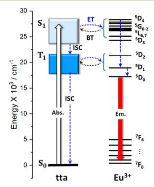
Fig. 7 Partial energy level diagram of the Bzim[Eu(tta) $_4$ ]  $\cdot$  H $_2$ O complex. The emission arises from the  $^5$ D $_0$  emitting level. S $_0$  and S $_1$  are the ligand ground and lowest singlet excited states, respectively. T $_1$  is the lowest triplet ligand level, Abs. is the initial absorption, ISC is the intersystem crossing, where Em. is the emission. ET and BT are the forward and backward energy transfer rates, respectively.
