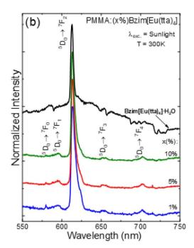
Fig. 6 Emission spectra of the Bzim[Eu(tta)<sub>4</sub>]  $\cdot$  H<sub>2</sub>O complex (black line) and the doped PMMA:(x%)Bzim[Eu(tta)<sub>4</sub>] polymers, where x = 1% (blue line), 5% (red line) and 10% (green line) with excitation at 380 nm (a) and under sunlight exposure (b). All spectra were recorded at room temperature in the range of 550 to 750 nm.
