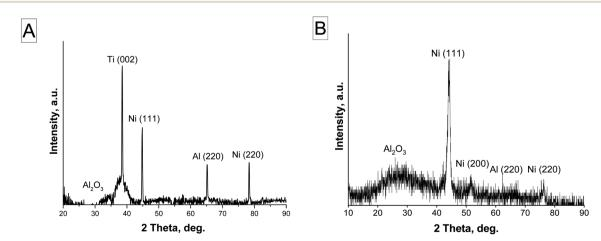
Fig. 5 XRD results of Ni-NPs electrodeposited in PAA: (A) variant 1, sample no. 1 (for the sample shown in Fig. 4A), (B) variant 2, sample no. 2 (for the sample shown in Fig. 4B).
