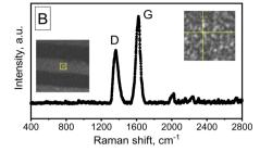
Fig. 8 Raman spectra ( $\lambda = 473$  nm) of MWCNTs for samples of two variants: (A) sample no. 1, (B) sample no. 2, measured at the location indicated in the photo, the inset shows surface SEM image of the experimental sample.
