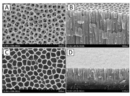
Fig. 3 Surface and cross-sectional SEM images of PAA obtained in the two-step mode of anodizing aluminum film for two variants of samples: (A and B) sample no. 1, after thinning the barrier layer, (C and D) sample no. 2, after barrier layer thinning and pores widening.
