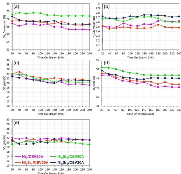
Fig. 6 Variation of (a) CH<sub>4</sub> conversion, (b) H<sub>2</sub>/CO molar ratio, (c) CO yield, (d) H<sub>2</sub> yield, and (e) CO<sub>2</sub> yield with time on stream for Ni<sub>5</sub>/CBV20A and Ni<sub>5</sub>Sr<sub>x</sub>/CBV20A (where  $x = 1-3$  wt%) catalysts at 700 °C and 1 atm (GHSV = 14 400 mL g<sup>-1</sup> h<sup>-1</sup>).
