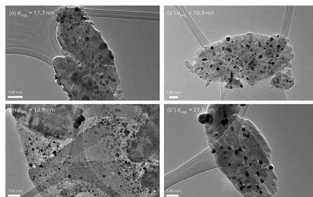
Fig. 9 TEM images and average particle size of (a) fresh Ni<sub>5</sub>/CBV20A, (b) used Ni<sub>5</sub>/CBV20A, (a') fresh Ni<sub>5</sub>Sr<sub>2</sub>/CBV20A and (b') used Ni<sub>5</sub>Sr<sub>2</sub>/CBV20A catalysts.
