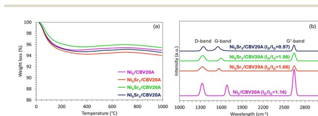
Fig. 8 (a) TGA profiles and (b) Raman spectra of the used Ni<sub>5</sub>/CBV20A and Ni<sub>5</sub>Sr<sub>x</sub>/CBV20A (where x = 1–3 wt%) catalysts.
