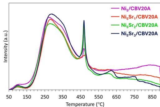
Fig. 4 CO<sub>2</sub>-TPD profiles of Ni<sub>5</sub>/CBV20A and Ni<sub>5</sub>Sr<sub>x</sub>/CBV20A (where x = 1–3 wt%) samples.
