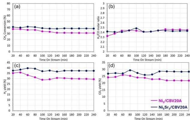
Fig. 7 Variation of (a) CH<sub>4</sub> conversion, (b) H<sub>2</sub>/CO molar ratio, (c) H<sub>2</sub> yield, and (d) CO<sub>2</sub> yield with time on stream for Ni<sub>5</sub>/CBV20A and Ni<sub>5</sub>Sr<sub>3</sub>/CBV20A catalysts at 700 °C and 1 atm (GHSV = 72 000 mL g<sup>-1</sup> h<sup>-1</sup>).
