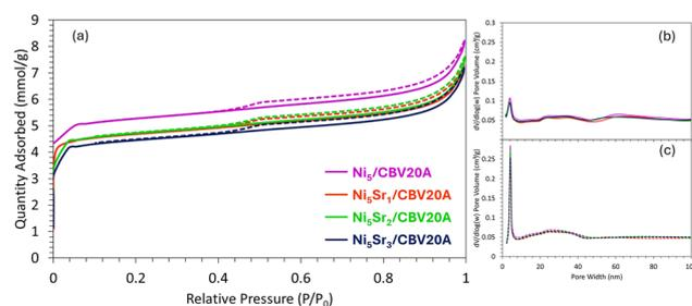
Fig. 1 (a) N<sub>2</sub> sorption isotherms and (b) adsorption and (c) desorption porosity distribution for fresh Ni<sub>5</sub>/CBV20A and Ni<sub>5</sub>Sr<sub>x</sub>/CBV20A (where x = 1–3 wt%) samples.
