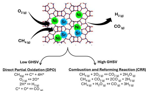
Fig. 10 Proposed reaction mechanism at low and high gas hourly space velocity.
