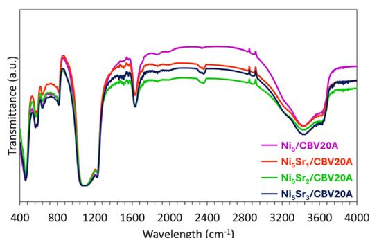
Fig. 5 FTIR spectra of Ni<sub>5</sub>/CBV20A and Ni<sub>5</sub>Sr<sub>x</sub>/CBV20A (where x = 1–3 wt%) samples.
