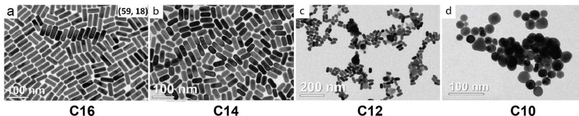
Fig. 13 Gold nanoparticles yielded from synthesis of a C<sub>n</sub>TAC : NaOL mixture with decreasing chain length (as indicated in the figure), leading to lower control of anisotropic growth and monodispersity.<sup>6</sup>
