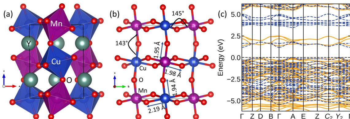
Fig. 5 (a) The optimized crystal structure and (b) distortion of  $\text{CuO}_6$  and  $\text{MnO}_6$  octahedra in YCMO; the Cu/Mn–O bond lengths and Cu–O–Mn bond angles are given. The significant difference between in-plane and out-of-plane Cu–O bonds indicates compression of the  $\text{CuO}_6$  octahedron. (c) The spin-polarized band structure in the FM state with PBE-DFT level of theory. The yellow (solid) and blue (broken) lines indicate major and minor spin channels, respectively.
