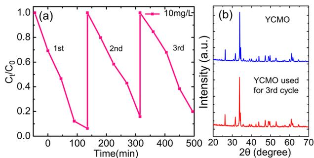
Fig. 9 (a) Recycle tests of the photocatalytic degradation of Rh-B solution over the YCMO double perovskite, and (b) comparison of the XRD patterns of the YCMO double perovskite before and after three successive photocatalytic degradation processes.
