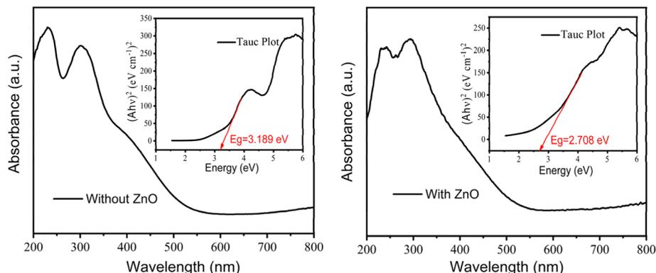
Fig. 10 UV-vis absorption spectrum of the coatings.
