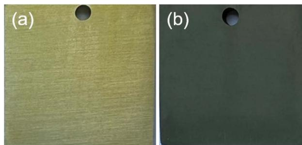
Fig. 1 Photos of specimen with conversion coating: without ZnO (a), with ZnO(b).
