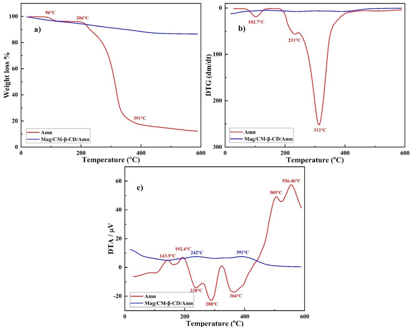
Fig. 5 (a) TG%, (b) DTG, and (c) DTA curves of Amn and Mag/CM-β-CD/Amn.
