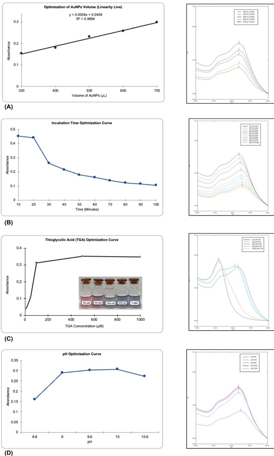
Fig. 2 UV-vis absorption spectra of different AuNPs volume (300, 400, 500, 600, 700  $\mu\text{L}$ ) (A); different incubation time (10, 20, 30, 40, 50, 60, 70, 80, 90, 100 minutes) (B) different TGA concentration 10, 50, 100, 500, 1000  $\mu\text{M}$  (C), and different pH (8.6, 9.0, 9.6, 10.0, 10.6) (D).
