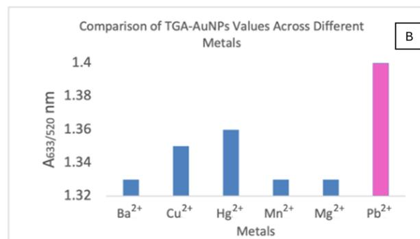
Fig. 5 Sensitivity in various Pb<sup>2+</sup> concentration (10, 1, 0.1, 0.01, 0.001  $\mu\text{g mL}^{-1}$ , and 0  $\mu\text{g mL}^{-1}$  control) (A) and selectivity (B) of the method for Pb<sup>2+</sup> detection when compared to different metal ions (Ba<sup>2+</sup>, Cu<sup>2+</sup>, Hg<sup>2+</sup>, Mg<sup>2+</sup>, Mn<sup>2+</sup>) at 9.5  $\mu\text{g mL}^{-1}$ .
