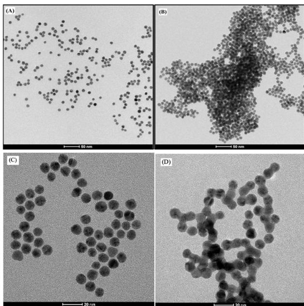
Fig. 3 TEM images of AuNPs (A), AuNPs-TGA/Pb<sup>2+</sup> (B) and HRTEM images of AuNPs (C), AuNPs-TGA/Pb<sup>2+</sup> (D) in the presence of 1  $\mu\text{M}$  Pb<sup>2+</sup>.
