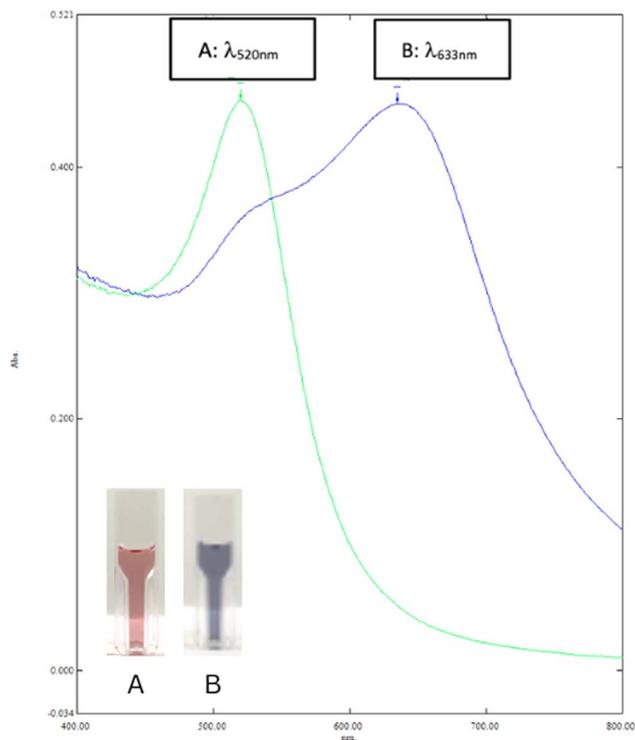
Fig. 1 UV-vis spectra of pre-treatment (A) of gold nanoparticles in water and post-treatment (B) of gold nanoparticles in the addition of 1 mL of pH 10.0 glycine–NaOH buffer, 50  $\mu\text{L}$  of 500  $\mu\text{M}$  TGA, and the presence of 50  $\mu\text{L}$  of 1  $\mu\text{M}$   $\text{Pb}^{2+}$ .
