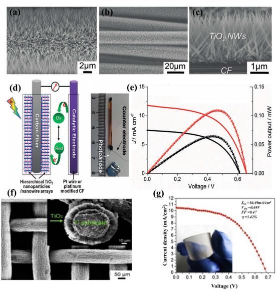
Fig. 10 (a–c) FESEM images of hierarchical  $TiO_2$  nanowire arrays grown over the CF substrate at 190 °C for 80 minutes, (d and e) schematic of wire DSSC consisting  $TiO_2$  nanoparticle and nanowires and Pt-modified CF counter electrodes and consequent J-V analysis, (f and g) low-magnification FESEM images of the  $TiO_2$  NWAs on Ti mesh substrates and respective J-V performance.<sup>72</sup>
