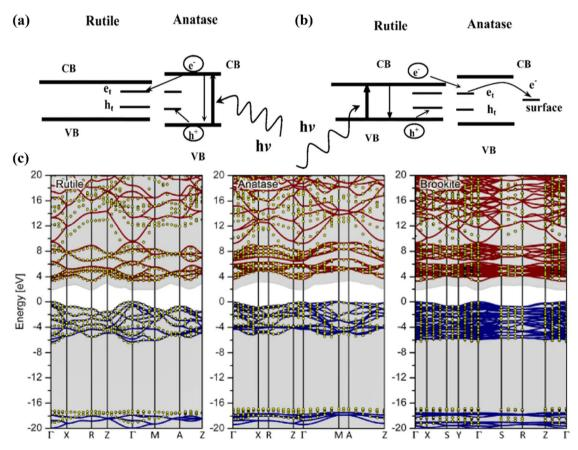
Fig. 7 (a and b) Typical schematics of charge trapping process in two-phase  $TiO_2$  namely rutile and anatase, which illustrate that photogenerated charges in the anatase phase can be further trapped *via* injection in the rutile phase, <sup>62</sup> (c) typical band structures and quasi-particle energies of different  $TiO_2$  phases (Rutile, Anatase, Brookite). <sup>63</sup>
