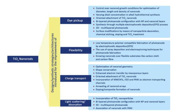
Fig. 12 Various modifications made in TiO<sub>2</sub> nanorods to improve the DSSCs performance.<sup>70</sup>
