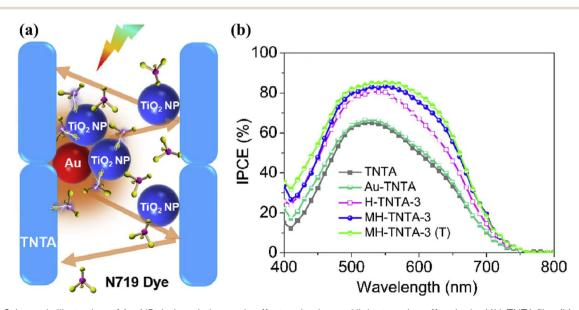
Fig. 16 (a) Schematic illustration of Au-NPs induced plasmonic effect and enhanced light-trapping effect in the MH-TNTA film, (b) consequent IPCE spectra of DSSCs based on various photoanodes. 103
