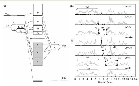
Fig. 17 (a) Detailed molecular orbital bonding diagram of  $TiO_2$  composed of the components extracted from the DOS spectra, <sup>112</sup> (b) density of states (DOS) of  $Ti_{1-x}A_xO_2$  doped *via* various metals (A: V, Cr, Mn, Fe, Co, Ni) where grey lines and black lines representing total DOS and dopant DOS respectively. <sup>113</sup>
