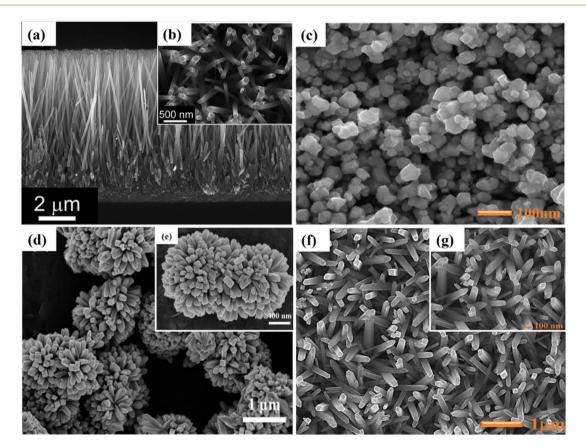
Fig. 4 Typical nanostructured FESEM images of various metal oxides that were generally used as a photoanode in DSSC applications. (a and b) ZnO-nanorods,<sup>35</sup> (c) Zn<sub>2</sub>SnO<sub>4</sub>-nanoparticles,<sup>36</sup> (d and e) SnO<sub>2</sub>-nanoflower,<sup>37</sup> and (f and g) TiO<sub>2</sub>-nanorods.<sup>38</sup>
