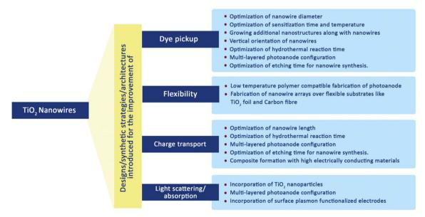
Fig. 9 Various modifications made in TiO<sub>2</sub> nanowires to improve the DSSCs performance.<sup>70</sup>
