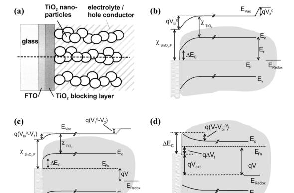
Fig. 18 (a) Schematic side view of a DSSC comprising nanocrystalline 1-D TiO<sub>2</sub> photoanodes and electrolyte, (b and c) schematic band model of DSSC under dark and light conditions, where the interfacial band bending arises due to the negative charges present in the electrolyte, and (d) detailed band diagram where light-induced V exceeds the  $V_{\rm bi}$ .
