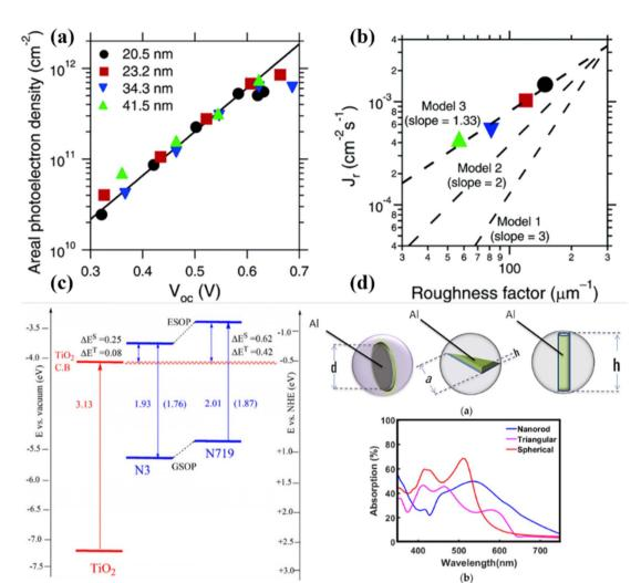
Fig. 3 Important features of photoanodes that can affect the DSSC performance significantly (a and b) photoanodes surface area and roughness-dependent photocurrent density, <sup>28</sup> (c) suitable bandgap alignment for better charge injection and transfer, <sup>29</sup> and (d) photoanode morphology-dependent tuning of light absorption capability, causing enhanced performance. <sup>30</sup>
