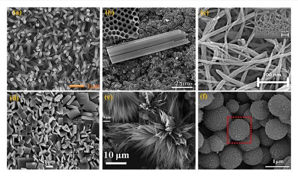
Fig. 6 FESEM images of various TiO<sub>2</sub> photoanodes including 1D, 2D and 3D structures explored for DSSC application. (a) Nanorods,<sup>38</sup> (b) nanotubes,<sup>57</sup> (c) nanowires,<sup>58</sup> (d) nanosheets,<sup>59</sup> (e) nanoflower,<sup>60</sup> and (f) nanoshere.<sup>61</sup>
