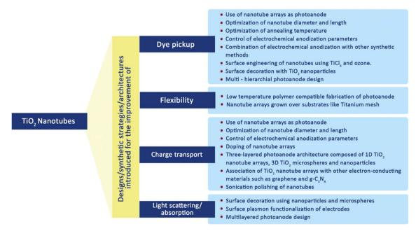
Fig. 14 Various modifications were made to the TiO<sub>2</sub> nanotubes to improve the DSSC's performance.<sup>70</sup>
