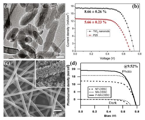
Fig. 13 (a and b) High resolution TEM image of single crystalline anatase  $TiO_2$  nanorods and the respective DSSC performance with 8.66% PCE, <sup>84</sup> (c and d) typical SEM image of electro-spun  $TiO_2$ -PVAs nanofibers with heat treated @400 °C SEM image in inset and their consequent performance with PCE of 9.52%. <sup>85</sup>
