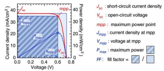
Fig. 2 Typical schematic representation of various J-V parameters to evaluate the solar cell performance.<sup>27</sup>
