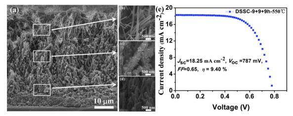
Fig. 11 (a) Cross-sectional FESEM image of TiO<sub>2</sub> nanowires grown on FTO substrate in 3 cycles of 9 h each, (b-d) FESEM images of top, intermediate, and bottom layers of grown nanowires, (e) J-V analysis of the DSSC prepared using these TiO<sub>2</sub> nanowires having total thickness of 47 μm.<sup>75</sup>
