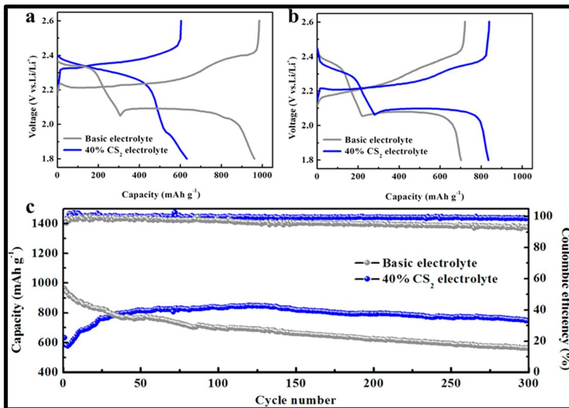
Fig. 9 Electrochemical performance of Li-S cells with basic and 40 wt% CS<sub>2</sub> electrolytes. (a) The initial charge–discharge voltage profiles at 0.5C rate. (b) The 100th charge–discharge profiles at 0.5C rate. (c) Cycle performance of Li-S cells with different electrolytes at 0.5C.<sup>74</sup>
