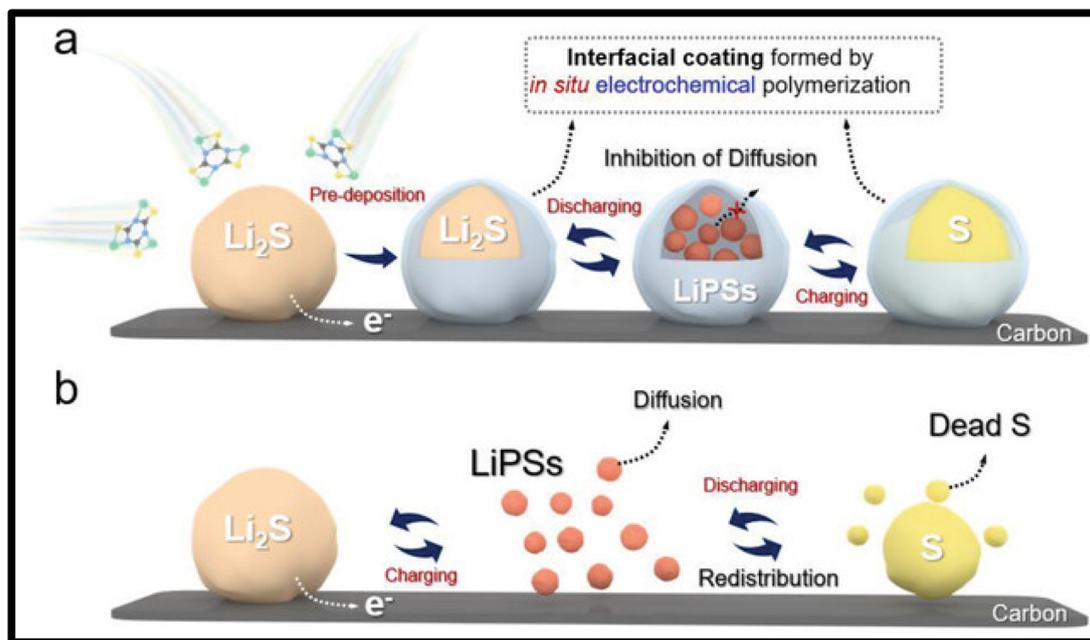
Fig. 8 Schematic of *in situ* coating Li<sub>2</sub>S with polymerizable electrolyte additive. (a) The soluble TTCA-Li electrochemically polymerizes on the Li<sub>2</sub>S surface to form a POS coating during the initial charging, which inhibits the out-diffusion of LiPSs during subsequent cycling. (b) Li<sub>2</sub>S cathodes without TTCA-Li additive generate soluble LiPSs and undergo uncontrollable sulfur redistribution during cycling.<sup>142</sup>
