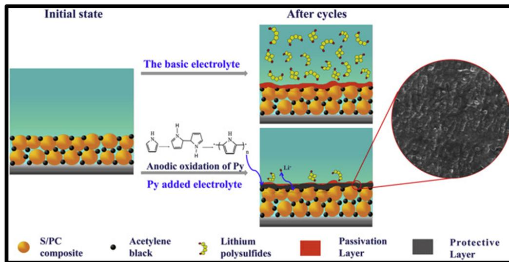
Fig. 10 Schematic illustration of the formed protective layer on the surface of sulfur cathode by adding pyrrole into the electrolyte.<sup>75</sup>
