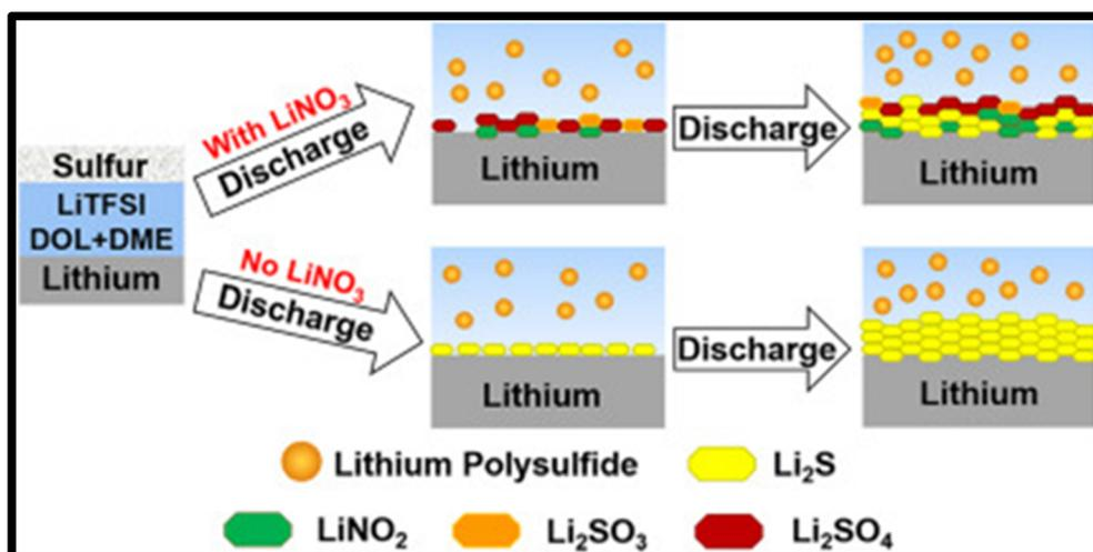
Fig. 2 Comparative mechanisms of SEI formation on lithium anodes with (top) and without (bottom) LiNO<sub>3</sub> additive in electrolytes.<sup>85</sup>
