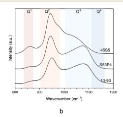
Fig. 2 Raman spectra of glasses 45S5, S53P4 and 13-93: (a) entire spectra and (b) high-frequency region only.
