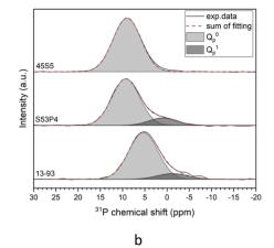
Fig. 1 (a)  $^{29}$ Si and (b)  $^{31}$ P MAS NMR spectra and their deconvolution for glasses 45S5, S53P4 and 13-93.
