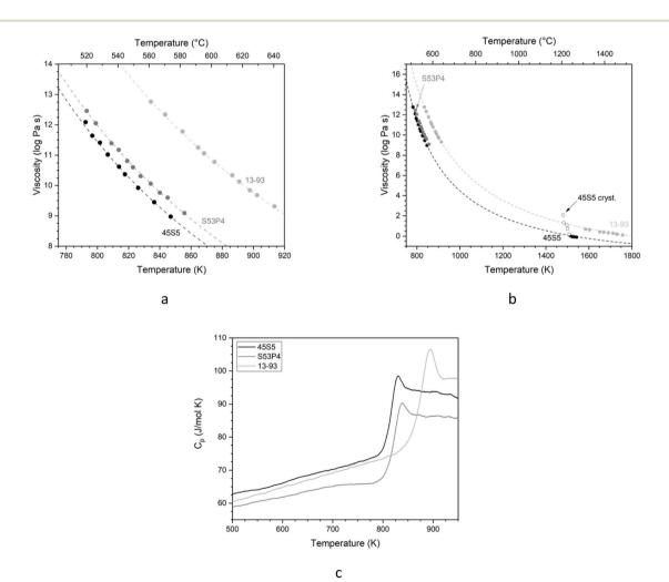
Fig. 3 Viscosity of the glasses as a function of temperature fitted with (a) the Vogel–Fulcher–Tammann equation for measurements at low temperatures and (b) the Adam–Gibbs equation for the entire temperature range. Symbols show experimental data points and dashed lines show fitting. Open symbols represent values for 45S5 with crystallisation occurring. (c) Molar heat capacity of the glasses, plotted over the temperature.
