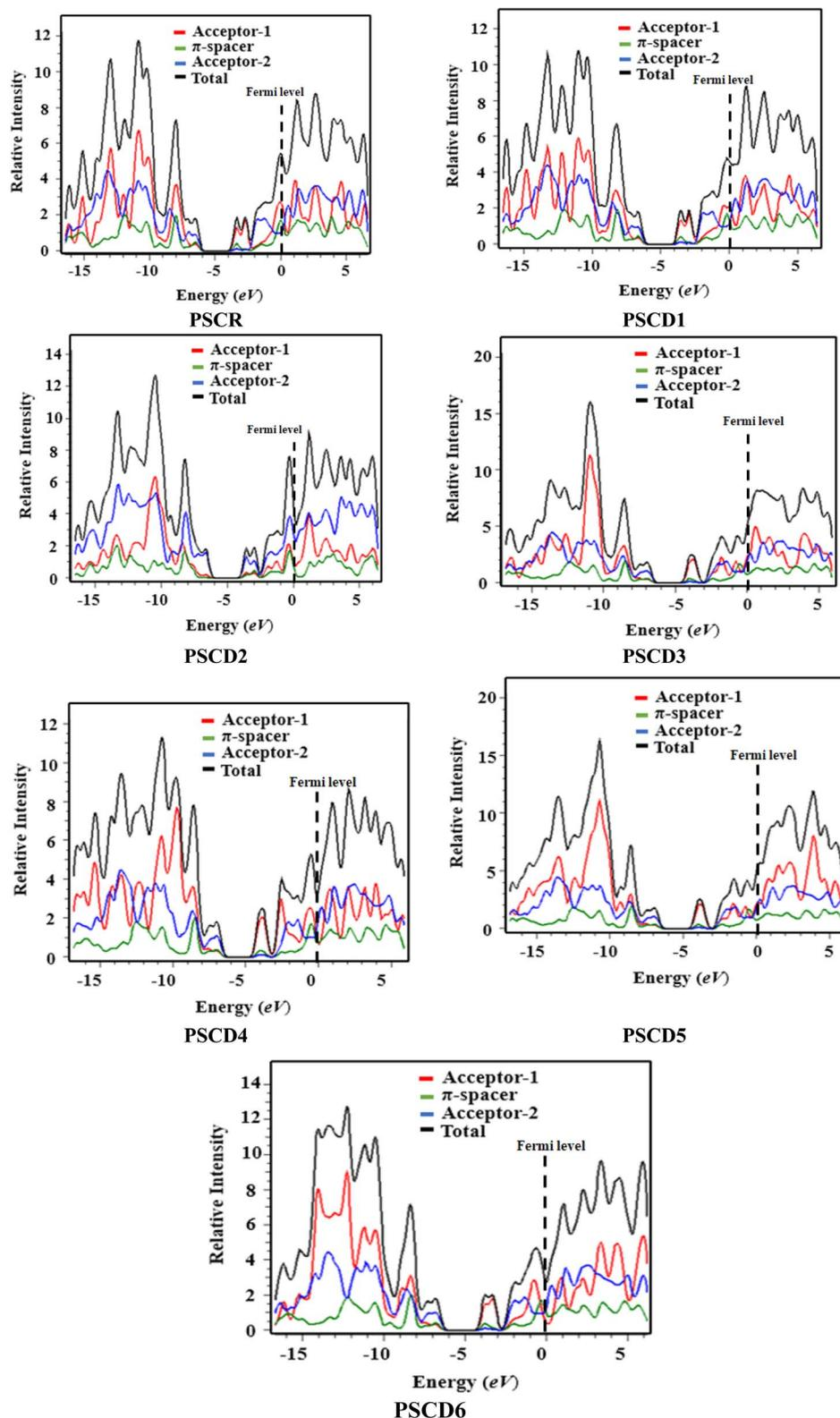
Fig. 4 DOS plots for PSCR and PSCD1–PSCD6.
