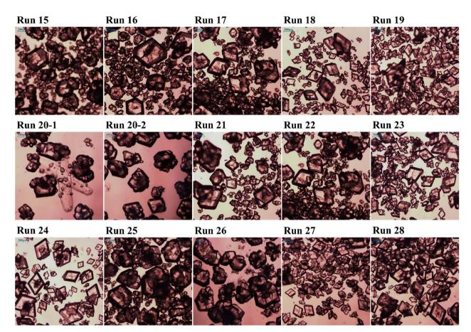
Fig. 6 OM image of LGA crystals using α-form seed in Table 2: Run 15 to Run 19 have different cooling rate, Run 20 to Run 24 have different supersaturation and Run 24 to Run 28 are about the effects of seed mass
