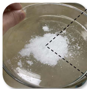
Fig. 9 OM image of a crystal being transferred to a Petri dish immediately after filtration, needle-like shape: looks like fiber, \alpha -form seeded (Run 25): looks like grain of salt.
