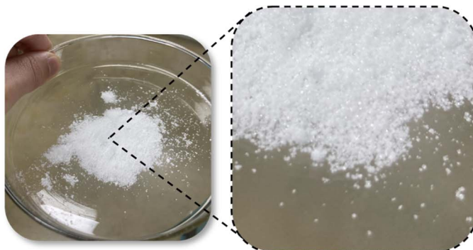
Fig. 9 OM image of a crystal being transferred to a Petri dish immediately after filtration, needle-like shape: looks like fiber, α-form seeded (Run 25): looks like grain of salt.
