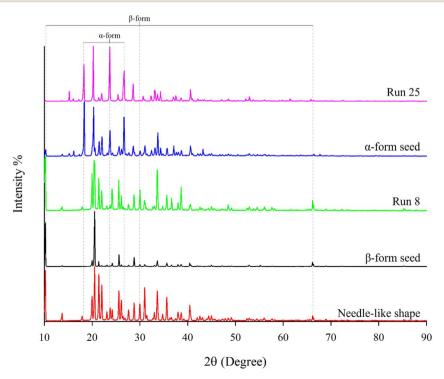
Fig. 7 XRD pattern – needle-like shape,  $\beta$ -form seed, Run 8,  $\alpha$ -form seed, Run 25.
