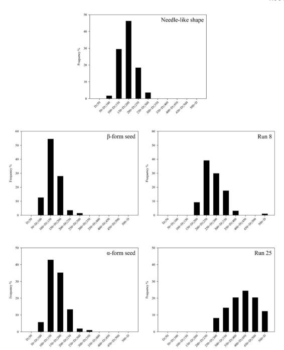
Fig. 11 Distribution of crystal diameter (x-axis: crystal diameter range).
