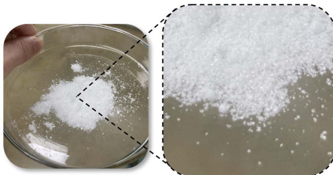
Fig. 9 OM image of a crystal being transferred to a Petri dish immediately after filtration, needle-like shape: looks like fiber, \alpha -form seeded (Run 25): looks like grain of salt.
