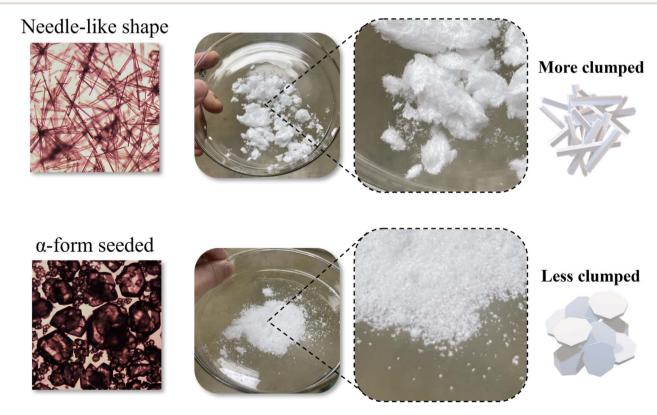
Fig. 9 OM image of a crystal being transferred to a Petri dish immediately after filtration, needle-like shape: looks like fiber,  $\alpha$ -form seeded (Run 25): looks like grain of salt.
