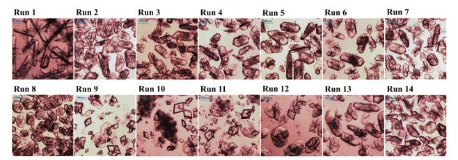
Fig. 5 OM image of LGA crystals using  $\beta$ -form seed in Table 2: Run 1 to Run 4 have different cooling rate, Run 5 to Run 8 have different supersaturation and Run 9 to Run 14 are about the effects of seed mass.
