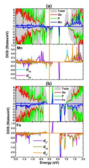
Fig. 8 Total density of states, atom-decomposed density of states, and projected density of states of transition metals calculated with PBE functional (vertical line: the Fermi level is set to 0 eV; positive DOS value: spin-up; negative DOS value: spin-down) of transition metal impurities in GeP monolayer doped with (a) single Mn atom (Mn<sub>Ge</sub> system) and (b) single Fe atom (FeGe system).
