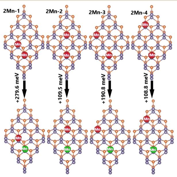
Fig. 11 Spin density (iso-surface value:  $0.02 \text{ e Å}^{-3}$ ; red surface: positive spin value; green surface: negative spin value) and energy of magnetic transition in 2Mn-n (n = 1, 2, 3, and 4) systems.
