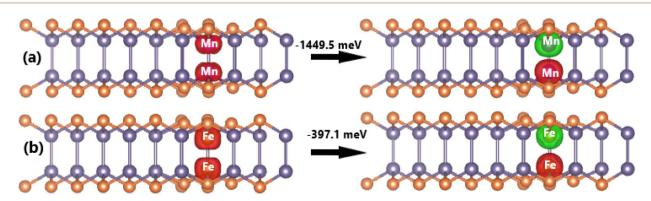
Spin density (iso-surface value:  $0.02 \text{ e } \text{Å}^{-3}$ ; red surface: positive spin value; green surface: negative spin value) and energy of magnetic state transition in (a) pMn- and (b) pFe-doped GeP monolayer.
