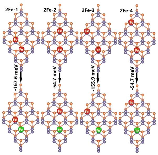
Fig. 12 Spin density (iso-surface value: 0.02 e Å<sup>-3</sup>; red surface: positive spin value; green surface: negative spin value) and energy of magnetic transition in 2Fe-n (n = 1, 2, 3, and 4) systems.
