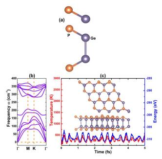
Fig. 1 (a) Atomic structure in a unit cell (top-view and side-view), (b) phonon dispersion curves, and (c) fluctuation of temperature and energy during AIMD simulations ((Inset): atomic structure after simulations), of GeP monolayer.
