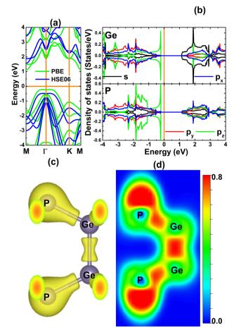
Fig. 2 (a) Electronic band structure (horizontal line: the Fermi level is set to 0 eV), (b) projected density of states calculated using the PBE functional (vertical line: the Fermi level is set to 0 eV; positive DOS value: spin-up; negative DOS value: spin-down), (c) charge distribution (iso-surface value:  $0.06 \, \mathrm{e} \, \mathrm{\mathring{A}}^{-3}$ ), and (d) electron localization function of the GeP monolayer.
