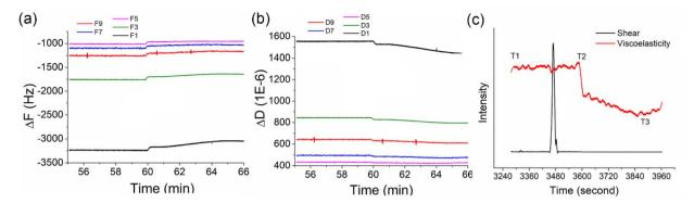
Fig. 4 (a) Resonant frequency and (b) energy dissipation of AZ1518 under 405 nm irradiation. (c) Shear and viscoelasticity of the photoresist
