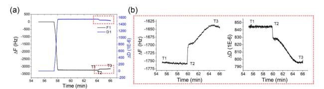
Fig. 3 (a) Real-time dynamic monitoring of the UV-induced photochemical reaction of AZ1518 on a QCM chip. (b) Plots of the frequency shift and energy dissipation of the photoresist under 405 nm irradiation.
