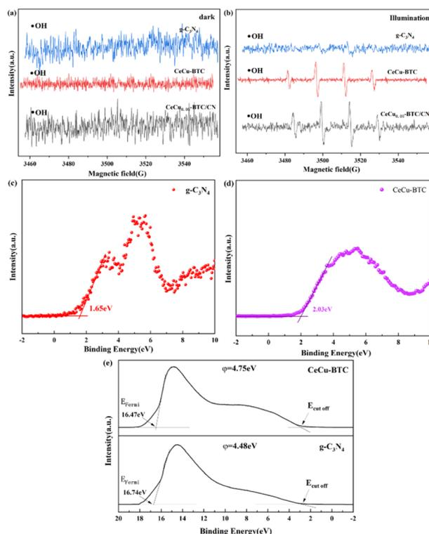
Fig. 7 EPR spectra of DMPO-<sup>•</sup>OH spin capture (a and b), VB-XPS (c and d), UV electron spectroscopy UPS (e).
