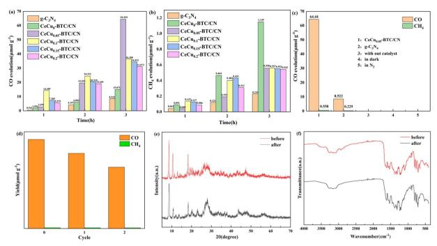
Fig. 6 Photocatalytic  $CO_2$  reduction CO yield plot (a),  $CH_4$  yield plot (b), control experiment (c),  $CeCu_{0.05}$ -BTC/CN cycle test (d), XRD and FT-IR changes of the samples before and after illumination (e and f).
