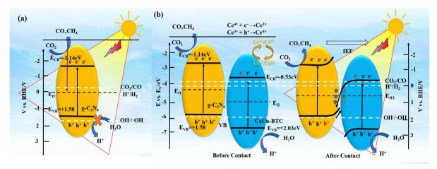
Fig. 8 Photocatalytic mechanism diagram of  $g-C_3N_4$  (a), the work functions of CN and CeCu-BTC before/after contact and the formation of internal electric field (b).
