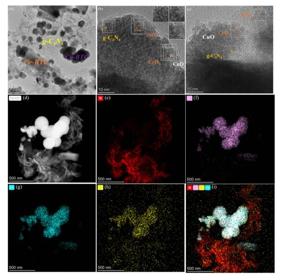
Fig. 3 TEM (HR-TEM) (a-c) of CeCu<sub>0.05</sub>-BTC/CN, dark field image of CeCu<sub>0.05</sub>-BTC/CN (d), EDS mapping image: N (e), O (f), Ce (g), Cu (h), general diagram of element distribution (i).
