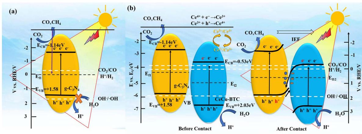
Fig. 8 Photocatalytic mechanism diagram of g-C<sub>3</sub>N<sub>4</sub> (a), the work functions of CN and CeCu-BTC before/after contact and the formation of internal electric field (b).
