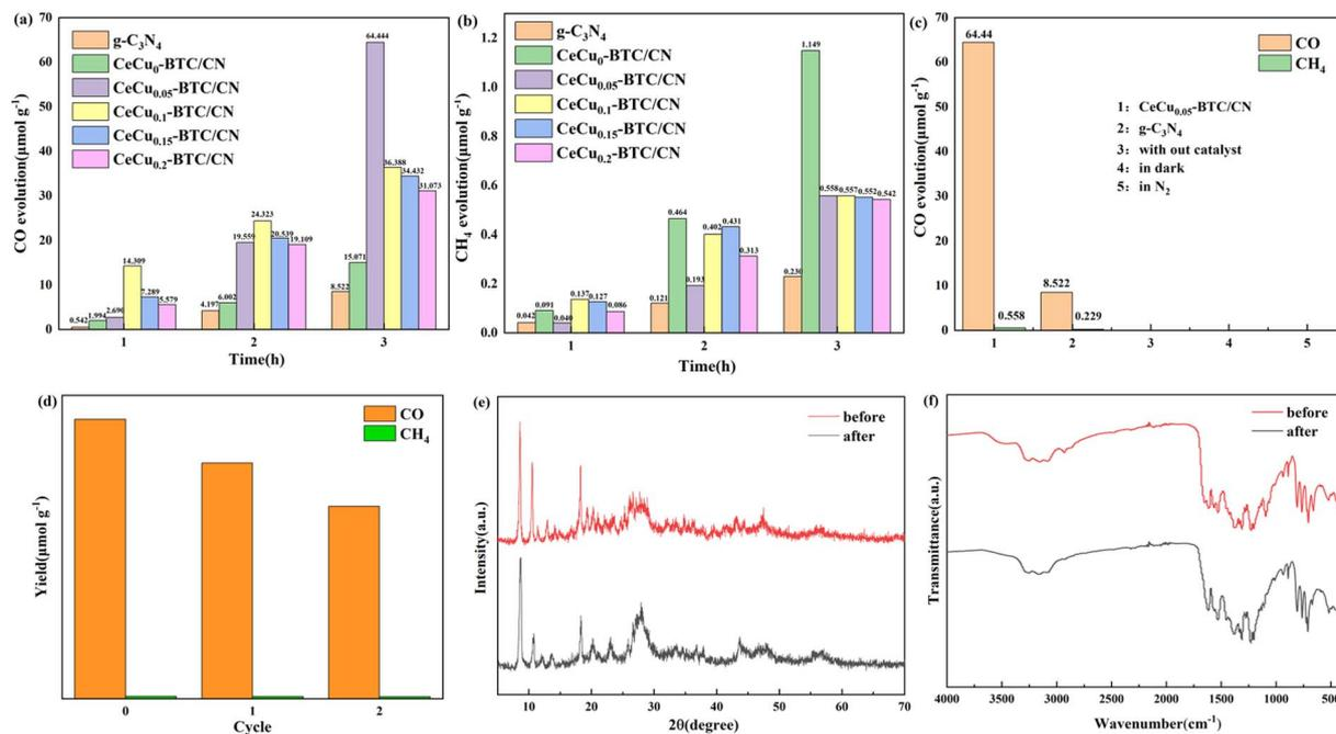
Fig. 6 Photocatalytic CO<sub>2</sub> reduction CO yield plot (a), CH<sub>4</sub> yield plot (b), control experiment (c), CeCu<sub>0.05</sub>-BTC/CN cycle test (d), XRD and FT-IR changes of the samples before and after illumination (e and f).
