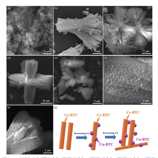
Fig. 2 SEM images of  $g-C_3N_4$  (a), Ce-BTC (b), CeCu $_0$ -BTC/CN (c), CeCu $_{0.05}$ -BTC/CN (d), CeCu $_{0.1}$ -BTC/CN (e), CeCu $_{0.05}$ -BTC/CN sample enlarged view (f), CeCu $_{0.1}$ -BTC/CN sample enlarged view (g), schematic diagram of sample crystal growth (h).
