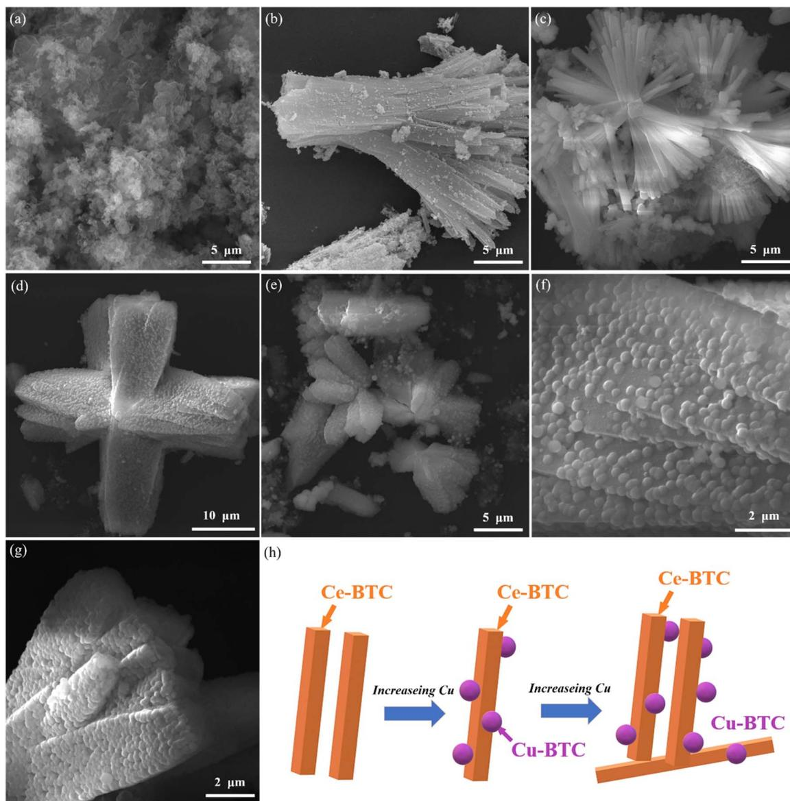
Fig. 2 SEM images of g-C<sub>3</sub>N<sub>4</sub> (a), Ce-BTC (b), CeCu<sub>0</sub>-BTC/CN (c), CeCu<sub>0.05</sub>-BTC/CN (d), CeCu<sub>0.1</sub>-BTC/CN (e), CeCu<sub>0.05</sub>-BTC/CN sample enlarged view (f), CeCu<sub>0.1</sub>-BTC/CN sample enlarged view (g), schematic diagram of sample crystal growth (h).
