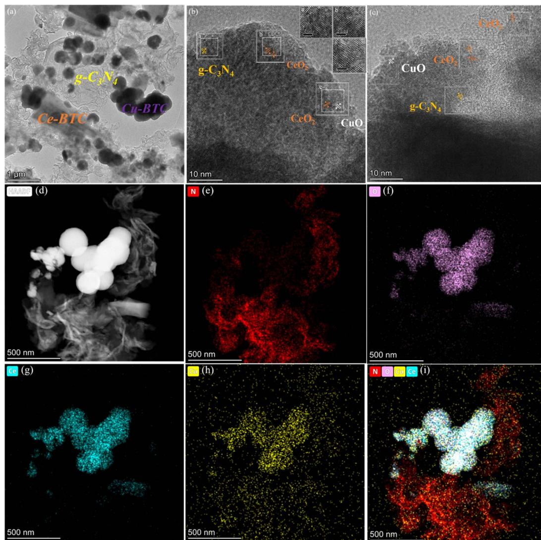
Fig. 3 TEM (HR-TEM) (a–c) of  $\text{CeCu}_{0.05}\text{-BTC/CN}$ , dark field image of  $\text{CeCu}_{0.05}\text{-BTC/CN}$  (d), EDS mapping image: N (e), O (f), Ce (g), Cu (h), general diagram of element distribution (i).
