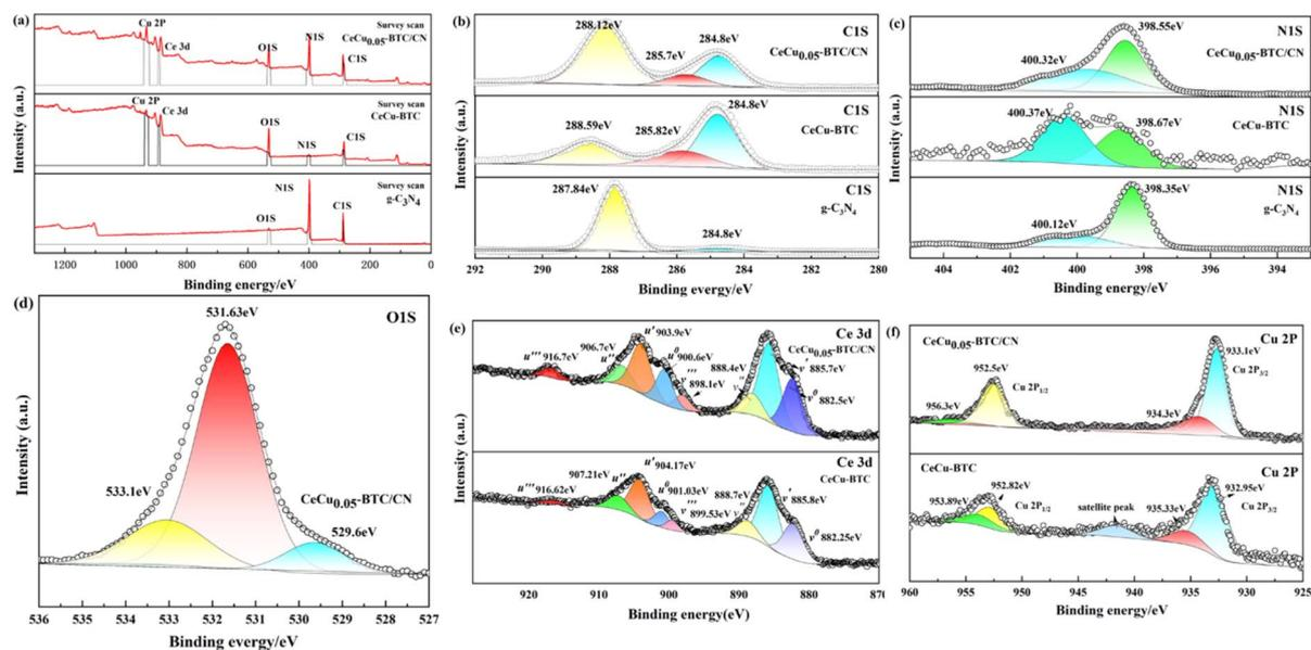
Fig. 4 XPS spectra of the  $g\text{-C}_3\text{N}_4$ , CeCu-BTC and CeCu<sub>0.05</sub>-BTC/CN: total elemental spectra (a), C 1s (b), N 1s (c) O 1s (d), Ce 3d (e), Cu 2p (f).
