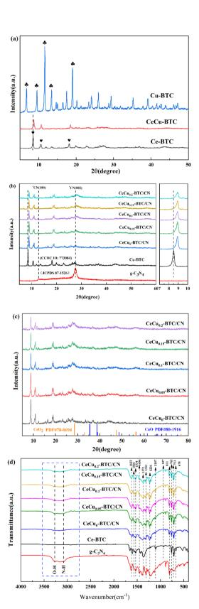
Fig. 1 XRD patterns of Ce-BTC, Cu-BTC and CeCu-BTC (a), g-C<sub>3</sub>N<sub>4</sub>, Ce-BTC and CeCu<sub>x</sub>-BTC/CN (b), XRD spectra of CeO<sub>2</sub> and CuO (c), FT-IR spectra of g-C<sub>3</sub>N<sub>4</sub>, Ce-BTC and CeCu<sub>x</sub>-BTC/CN (d).
