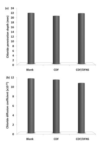
Fig. 16 Chloride penetration depth (a) and diffusion coefficient (b) at a 21-day rehabilitating age.
