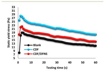
Fig. 8  $\,$  Analysis of the role of CDF and CDF/DFNS in the elastic limit of cement paste.
