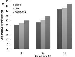
Fig. 14 Role of CDF and CDF/DFNS in (a) bending rigidity, (b) compressive force of cement at the recovery generation of 21 days.
