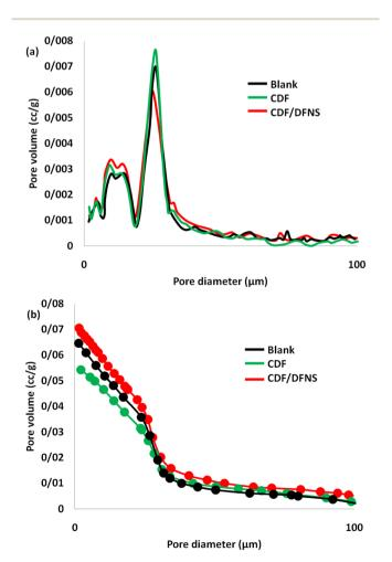
Fig. 12 The distribution of opening measurements (a), and cumulative opening volume of cement healed at 21 days >200 (b).
