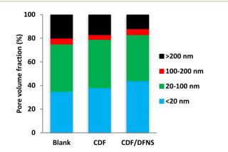
Fig. 13 Vent volume fraction of cement healed at 21 days.
