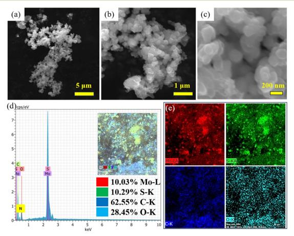
Fig. 3 (a-c) Low- to high-magnification FESEM images of PPy/MoS<sub>2</sub>. (d and e) EDAX and elemental mapping of PPy/MoS<sub>2</sub>.
