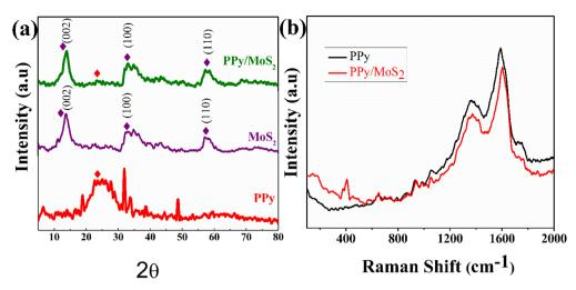
Fig. 2 (a) XRD of PPy, MoS<sub>2</sub> and PPy/MoS<sub>2</sub>. (b) Raman spectra of PPy and PPy/MoS<sub>2</sub>.
