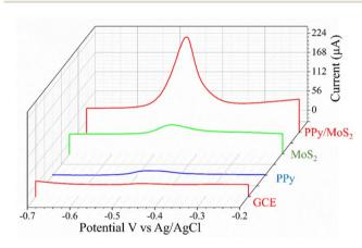
Fig. 5 SWASV comparison of GCE, PPy, MoS<sub>2</sub> and PPy/MoS<sub>2</sub> electrodes for the detection of 300 nM Pb<sup>2+</sup> concentration.
