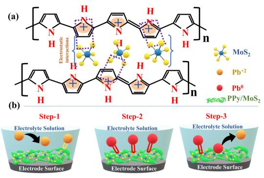
Fig. 1 (a) Possible functionalization mechanism of MoS<sub>2</sub> into the PPy polymer skeleton. (b) Schematic illustration of SWASV for detection of Pb $^{2+}$ by PPy/MoS<sub>2</sub> sensor.
