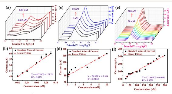
Fig. 6 (a) SWASV detection of  $Pb^{2+}$  with a range of 0.02 to 0.09 nM and (b) its respective calibration plot. (c) SWASV detection of  $Pb^{2+}$  with a range of 1 to 10 nM and (d) its respective calibration plot. (e) SWASV detection of  $Pb^{2+}$  with a range of 20 to 300 nM and (f) its respective calibration plot, under optimal SWASV experimental conditions.
