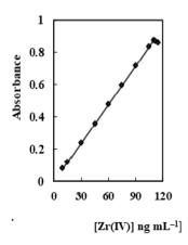
Fig. 6 Calibration curve for Zr(v) using the proposed PIM sensor at the optimum conditions.
