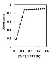
Fig. 4 Molar ratio method for the complexation of  ${\rm Zr}^{4+}$  and BTAHQ ant the optimum conditions.
