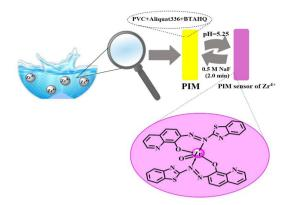
Scheme 2 Schematic representation for the preparation and complexation of Zr(v) ions on the formed optical sensor.
