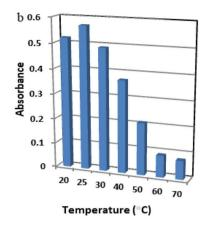
Fig. 2 Effect of (a) Aliquat 336 and (b) temperature on the PIM based sensor immersed in 60 ng mL $^{-1}$  of Zr(v) at the optimum conditions.
