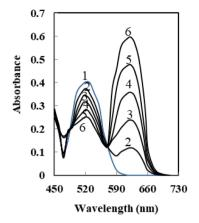
Fig. 1 Absorption spectra of 1- BTAHQ membrane and PIM based sensor upon contact with (2-6), 15, 30, 45, 60, and 75 ng per mL Zr(IV) at pH 5.25.
