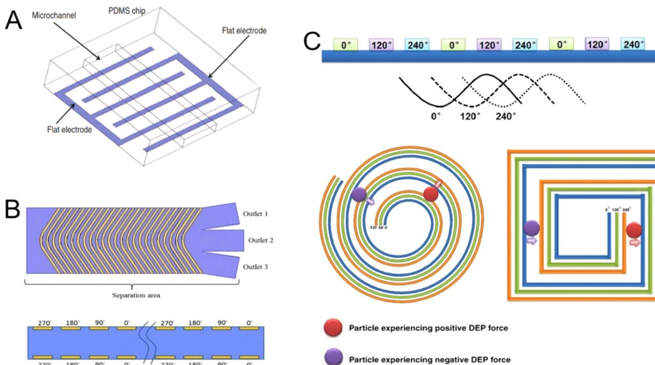
Fig. 11 DEP structural design for biological applications. (A) Schematic of electrodes.<sup>158</sup> (B) A chevron electrode configuration eliminating the erratic electric field and unexpected DEP and twDEP behaviours of the cells.<sup>159</sup> (C) Spiral electrode array intended to create an electric field phase gradient in a three-phase travelling-wave DEP system.<sup>160</sup>
