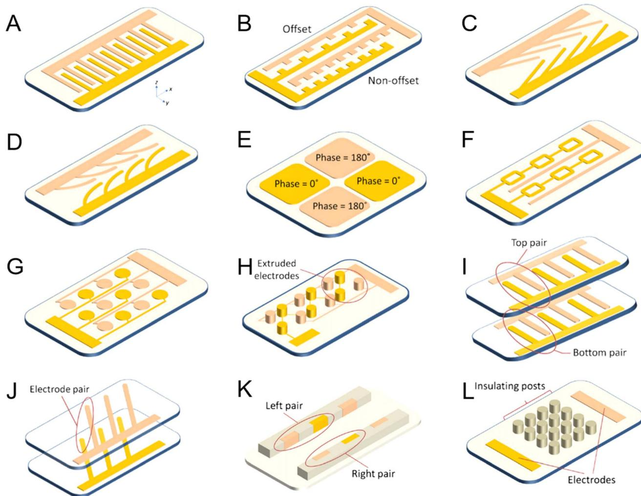
Fig. 8 DEP devices categorized based on the arrangement of microelectrodes:<sup>112</sup> (A) parallel or intersecting, (B) cylindrical, (C) angled, (D) curved, (E) quadrupole, (F) microporous, (G) matrix, (H) extruded, (I and J) top-down pattern, (K) sidewall pattern, and (L) insulator-based or nonpolar.
