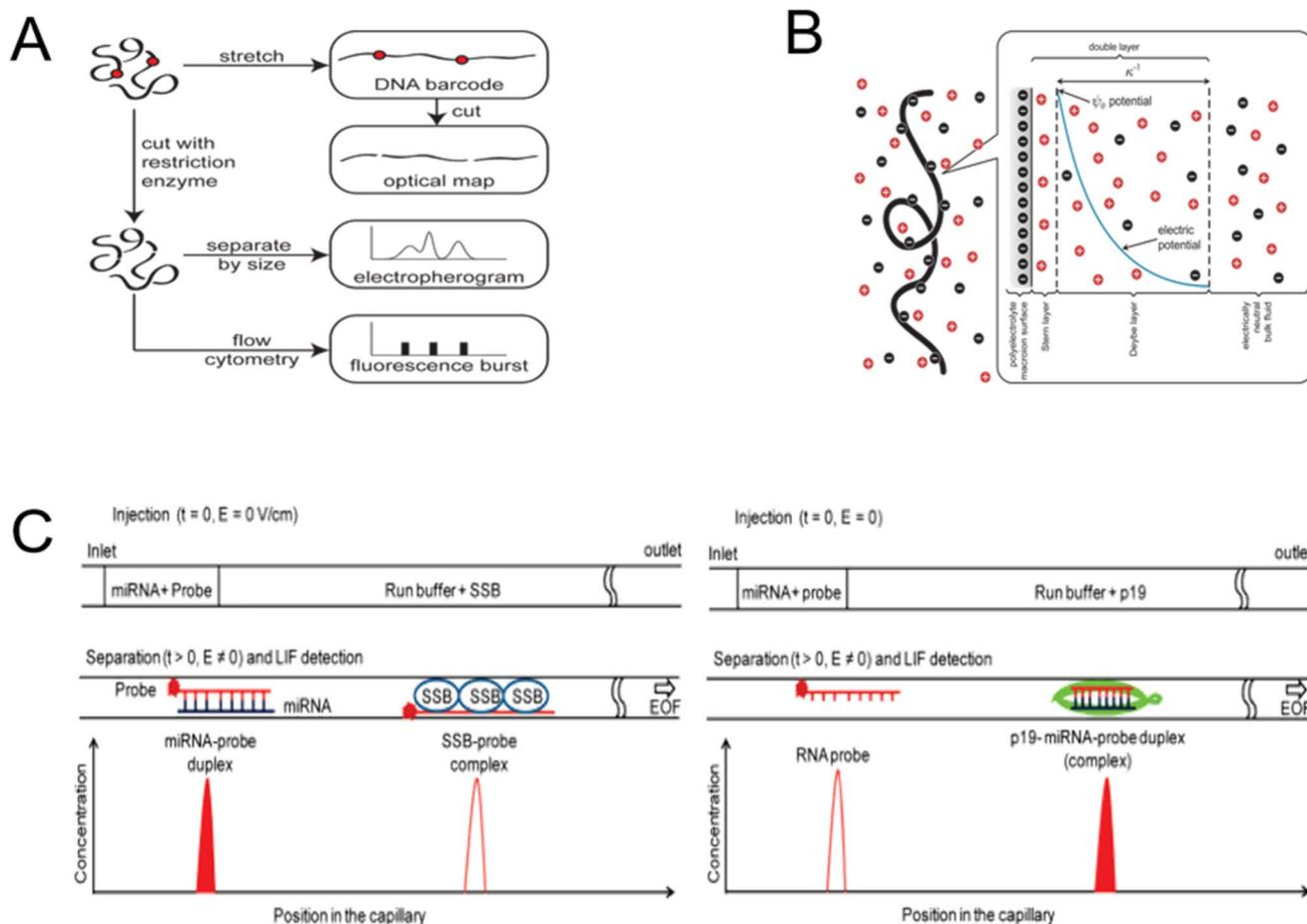
Fig. 3 Detection and separation of DNA using capillary electrophoresis. (A) The chip is made up of a chamber with inlets and a network of microchannels for CE analysis.<sup>38</sup> (B) Diagram of the local electrostatics in the vicinity of a free-solution DNA coil.<sup>39</sup> (C) The protein-facilitated affinity capillary electrophoresis (ProFACE) is used to detect miRNA.<sup>40</sup>
