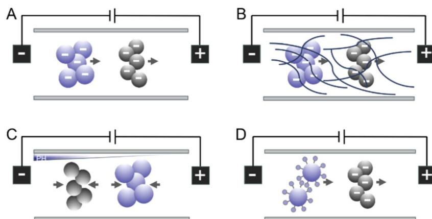
Fig. 2 Electrophoresis modes used in microsystems: (A) free solution electrophoresis. (B) Gel electrophoresis. (C) Isoelectric focusing. (D) Micellar electrokinetic chromatography (with negatively charged analytes depicted).<sup>25</sup>
