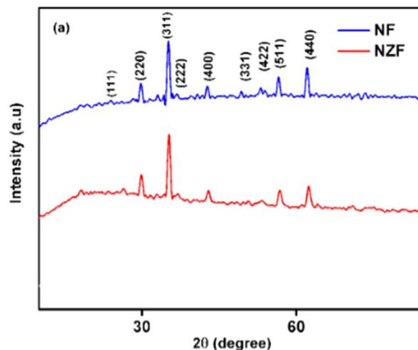
Fig. 1 X-ray diffraction patterns of nickel ferrite (NF) and  $Ni_{0.5}Zn_{0.5}Fe_2O_4$  (NZF) nanoparticles.
