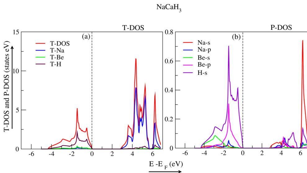
Fig. 6 Total and partial density of states for NaCaH<sub>3</sub>.
