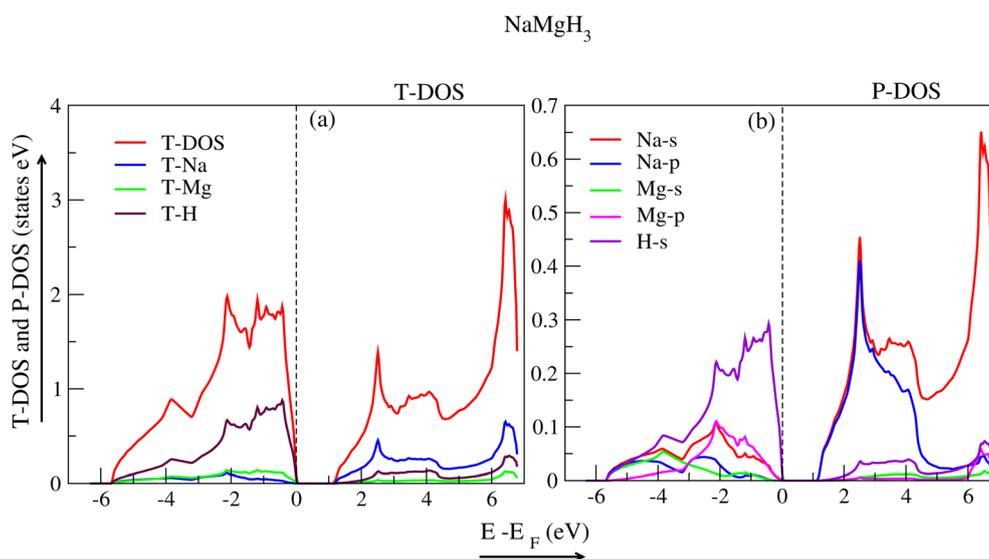
Fig. 7 Total and partial density of states for NaMgH<sub>3</sub>.
