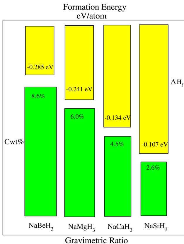
Fig. 3 Formation energy  $\Delta H_f$  (yellow bars) and gravimetric storage capacity  $C_{wt\%}$  (green bars) of NaXH<sub>3</sub> (X = Be, Mg, Ca, Sr).
