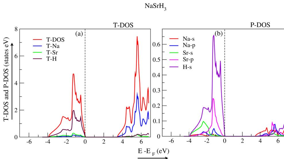
Fig. 8 Total and partial density of states for NaSrH<sub>3</sub>.
