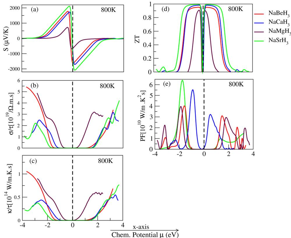
Fig. 9 Thermoelectric properties of NaXH<sub>3</sub> (X = Be, Mg, Ca, Sr).
