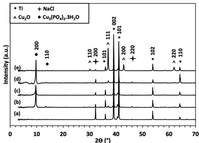
Fig. 7 XRD patterns of (a) NT-Control, (b) Ti/Cu 60, (c) NT/Cu 30, (d) NT/Cu 60, and (e) NT/Cu 90 after immersion in DPBS at  $37^\circ\text{C}$  for 24 hours.
