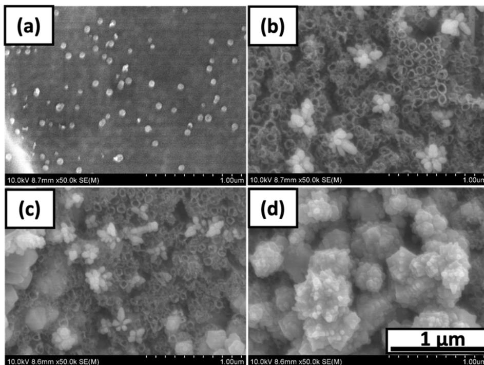
Fig. 2 SEM images of (a) Ti/Cu 60, (b) NT/Cu 30, (c) NT/Cu 60, (d) NT/Cu 90 after removal of top layer with tape.
