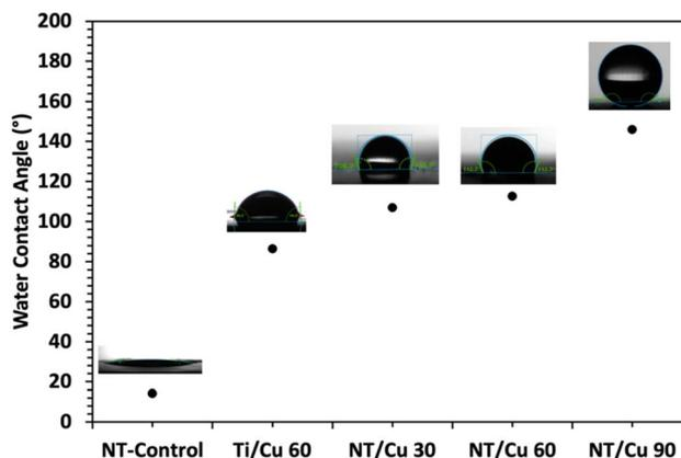
Fig. 5 Water contact angles of control surfaces.
