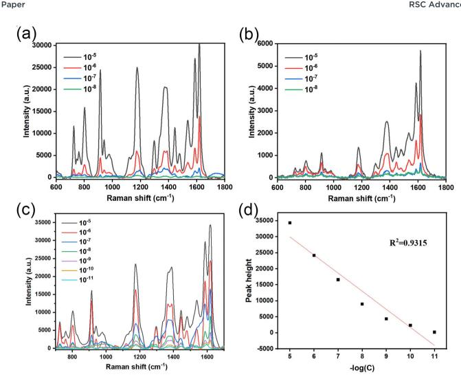
(a) – (c) respectively show the detection on different concentrations of CV solutions by use of the AgNPs/CuNPs/PSi substrate, the AuNPs/ CuNPs/Bragg-PSi substrate and the AgNPs/CuNPs/Bragg-PSi substrate. (d) Shows the linear fitting between the negative logarithm of the AgNPs/CuNPs/Bragg-PSi substrate for the CV solution concentration and the linear fitting degree of its Raman peak intensity at  $1617 \, \mathrm{cm}^{-1}$ .
