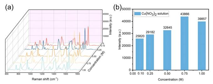
Fig. 4 (a) shows SERS spectra of  $10^{-5}$  M CV solution soaked in different concentrations of Cu(NO<sub>3</sub>)<sub>2</sub> solution; (b) shows the relationship between the concentration of Cu(NO<sub>3</sub>)<sub>2</sub> solution and its Raman peak intensity at 1617 cm<sup>-1</sup>.
