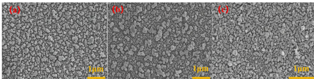
Fig. 2 (a) AgNPs/CuNPs/PSi; (b) AgNPs/CuNPs/Bragg-PSi; (c) AuNPs/CuNPs/Bragg-PSi.
