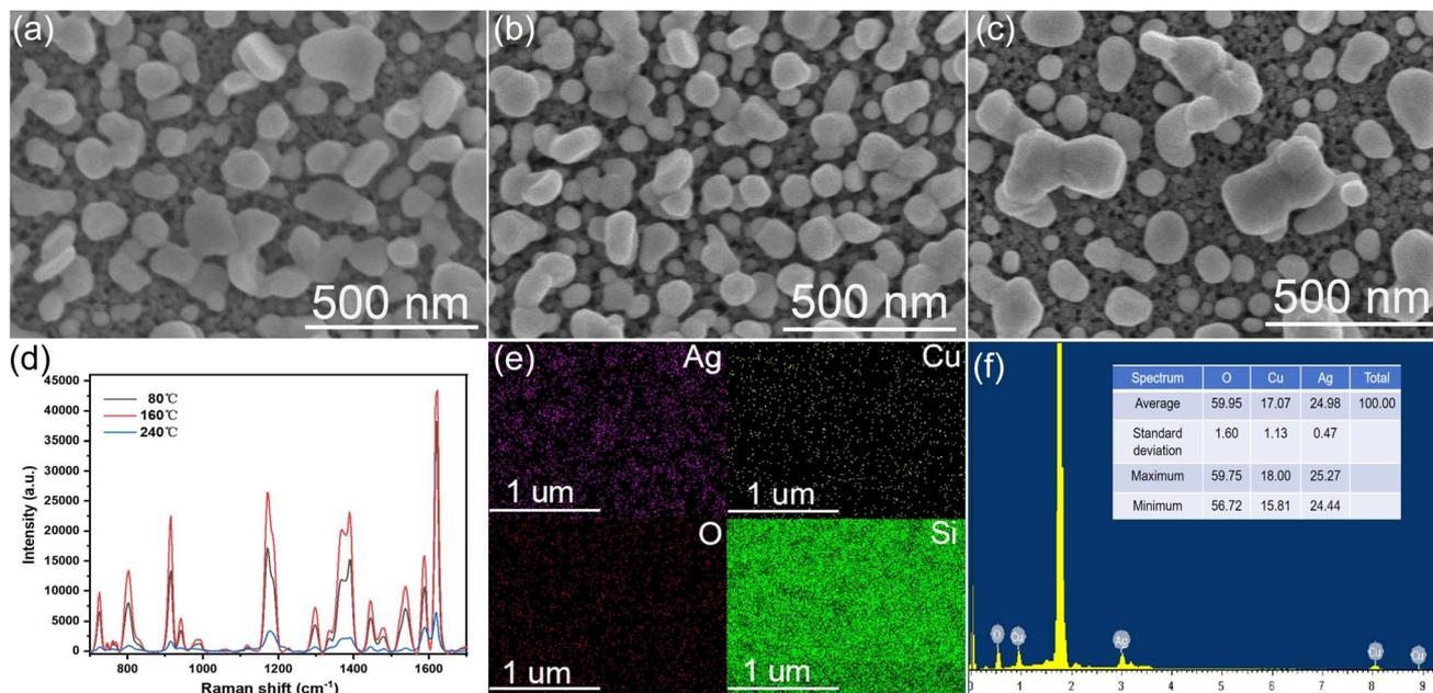
Fig. 5 (a–c) show SEM images of AgNPs/CuNPs/Bragg-PSi substrates annealed at 80 °C, 160 °C and 240 °C; (d) SERS spectra of AgNPs/CuNPs/Bragg-PSi substrates after annealing treatments at 80 °C, 160 °C, and 240 °C for  $10^{-5}$  M CV solution; (e) mapping image of AgNPs/CuNPs/Bragg-PSi substrate after annealing at 160 °C; (f) shows EDS energy spectra of annealed AgNPs/CuNPs/Bragg-PSi substrates.
