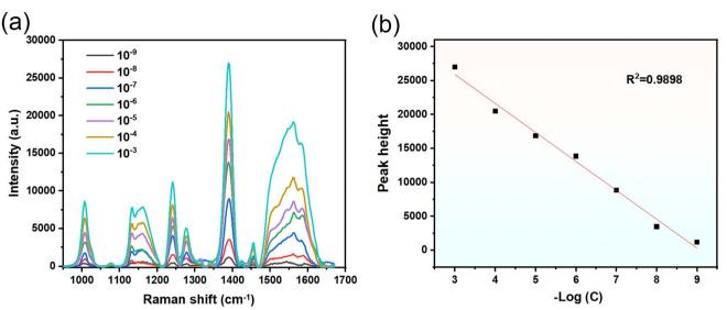
Fig. 8 (a) shows SERS spectrum of  $10^{-3}$ – $10^{-9}$  M diphenyl phthalate (DPHP); (b) shows linear fitting of the negative logarithm of the AgNPs/ CuNPs/Bragg-PSi substrate to the DPHP solution concentration and its Raman peak intensity at  $1388~{\rm cm}^{-1}$
