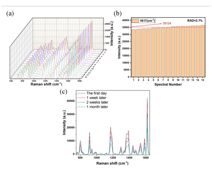
Fig. 7 (a) Randomly record the SERS spectra of 15 points of the CV solution; (b) the distribution of peak intensity at 1617 cm<sup>-1</sup> for the SERS spectra of 15 randomly selected CV solutions, with the green line representing the average intensity; (c) the relationship between the SERS signal intensity of AgNPs/CuNPs/Bragg-PSi substrates and their storage time.
