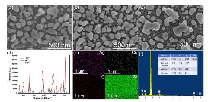
Fig. 5 (a-c) show SEM images of AqNPs/CuNPs/Bragg-PSi substrates annealed at 80 °C, 160 °C and 240 °C; (d) SERS spectra of AqNPs/CuNPs/ Bragg-PSi substrates after annealing treatments at 80 °C, 160 °C, and 240 °C for 10<sup>-5</sup> M CV solution; (e) mapping image of AgNPs/CuNPs/Bragg-PSi substrate after annealing at 160 °C; (f) shows EDS energy spectra of annealed AgNPs/CuNPs/Bragg-PSi substrates.
