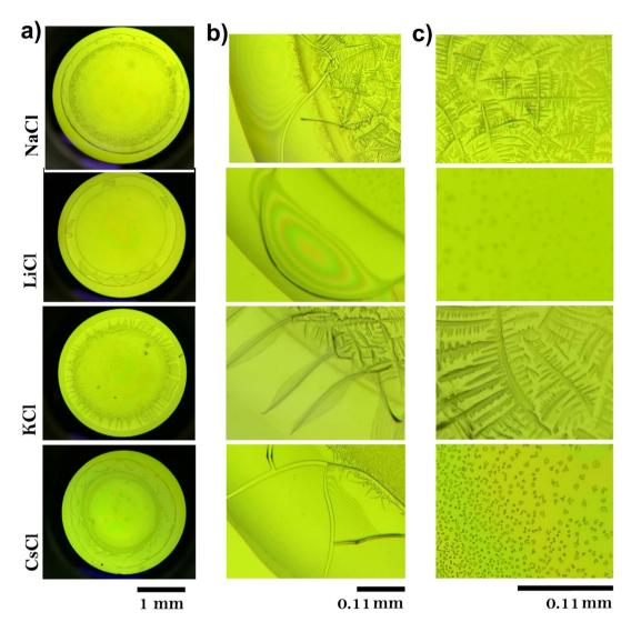
Fig. 5 Dried droplets of BSA suspensions with different salts. (a) Deposit patterns produced by NaCl, LiCl, KCl, and CsCl (C = 75 mM and  $C_p = 120$ μM). (b) The coffee ring of the deposits patterns. (c) A zoom of the central region in the deposits.
