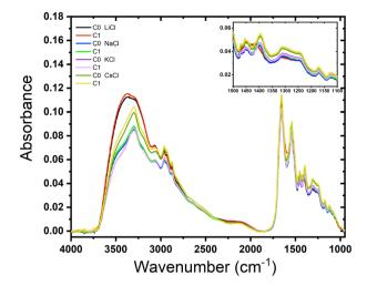
Fig. 4 Effect of rehydration of BSA films containing different salts. Absorbance as a function of the wave number of BSA films ( $C_p = 120 \, \mu M$  (8 mg mL<sup>-1</sup>)) with salts: LiCl, NaCl, KCl and CsCl ( $C = 75 \, \text{mM}$ ).
