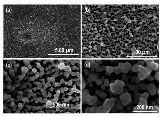
Fig. 5 FESEM images showing the morphology produced on the surface of Zr-4 as a result of chemical polishing for 5 min in HF:  $HNO_3$ :  $H_2O$  electrolyte (CP-5min-HFHNO $_3$ ) (a and b) low magnification images revealing the formation of columnar morphology, (c and d) high magnification images exhibiting the formation of nanostructure.
