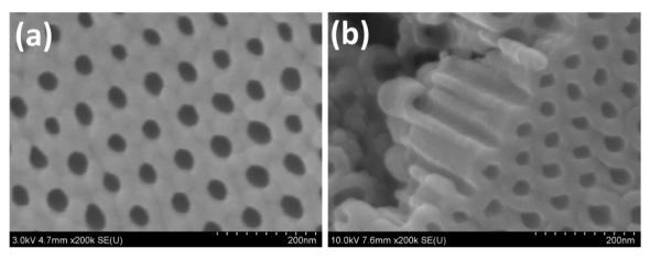
Fig. 10 FESEM images of the electropolished and anodized Zr-4 sample showing the (a) top surface view, (b) cross-sectional view of the Zr-4 oxide nanotubes.
