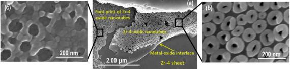
Fig. 12 FESEM images showing the (a) area near the metal-oxide interface in the Zr-4 substrate, (b) formation of Zr-4 oxide nanotubes with spacing. (c) foot pattern of Zr-4 oxide nanotubes after detachment as a result of sonication.
