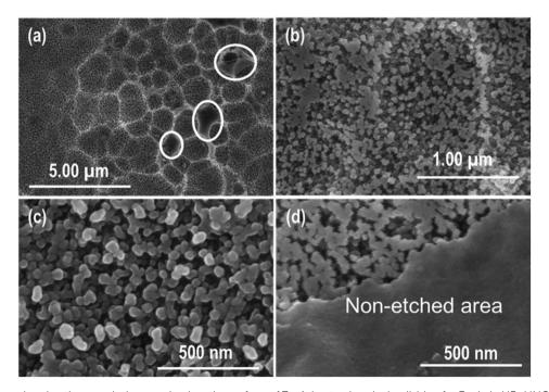
Fig. 4 FESEM images showing the morphology evolved on the surface of Zr-4 due to chemical polishing for 3 min in HF: HNO<sub>3</sub>: H₂O electrolyte (CP-3min-HFHNO<sub>3</sub>). (a and b) Low magnification images reveal the formation of grain boundaries, (c) high magnification images exhibit the formation of nanostructure inside the grains, and (d) high magnification images show the un-etched area of the Zr-4 sheet.
