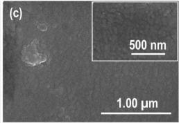
Fig. 1 (a) Digital picture of the as-received and mechanically polished Zr-4 sheet, FESEM images showing the morphology of the (b) as-received Zr-4 sheet, (c) mechanically polished Zr-4 sheet (MP-4000-45min).
