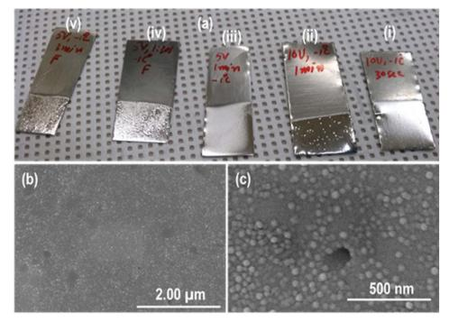
Fig. 2 (a) Digital picture of the electropolished Zr-4 sheet in methanol-perchloric acid (EP-MeOH-5V-1min, EP-MeOH-10V-30s, EP-MeOH-10V-1min, EP-MeOH-10V-3min), (b and c) FESEM images showing the morphology of the electropolished Zr-4 sheet.
