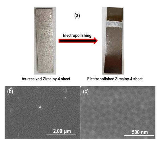
Fig. 3 (a) Digital picture of the as-received and electropolished Zr-4 sheet in ethylene glycol monobutyl ether-perchloric acid (EP-EG-50V-3°C-30min, EP-EG-50V-3°C-1min) (b and c) FESEM images showing the formation of a novel nanoscale patterned morphology on the surface of Zr-4 sheet after EP.
