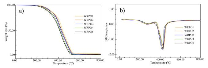
Fig. 5 TGA results of WRPOs: (a) TGA curves, (b) DTG curves
