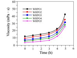
Fig. 2 Viscosity change curves of WRPOs versus time: WRPO1 (10% DCOA content), WRPO2 (20% DCOA content), WRPO3 (30% DCOA content), WRPO4 (35% DCOA content), and WRPO5 (40% DCOA content).
