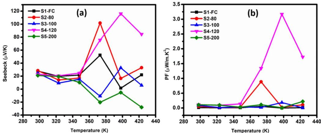
Fig. 5 Temperature dependent Seebeck coefficient (a) and thermoelectric power factor (PF) (b) of as-deposited functionalized multi-walled carbon nanotubes (F-MWCNTs) film and functionalized multi-walled carbon nanotubes (F-MWCNTs) films subject to hot-pressing at temperatures 80 °C, 100 °C, 120 °C, and 200 °C.
