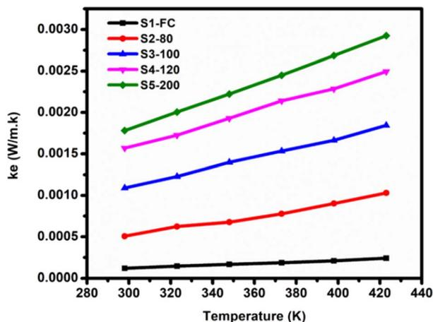
Fig. 6 Temperature dependent electronic thermal conductivity ( $k_e$ ) of as-deposited functionalized multi-walled carbon nanotubes (F-MWCNTs) film and functionalized multi-walled carbon nanotubes (F-MWCNTs) films subject to hot-pressing at temperatures 80 °C, 100 °C, 120 °C, and 200 °C.
