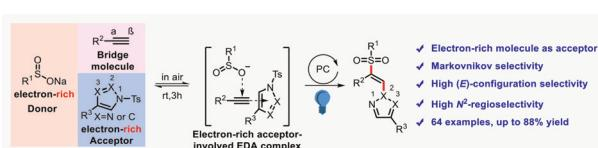
**A photocatalytic electron-rich acceptor-involved EDA complexes for Markovnikov addition of alkynes with *N*-sulfonyl-azoles**
