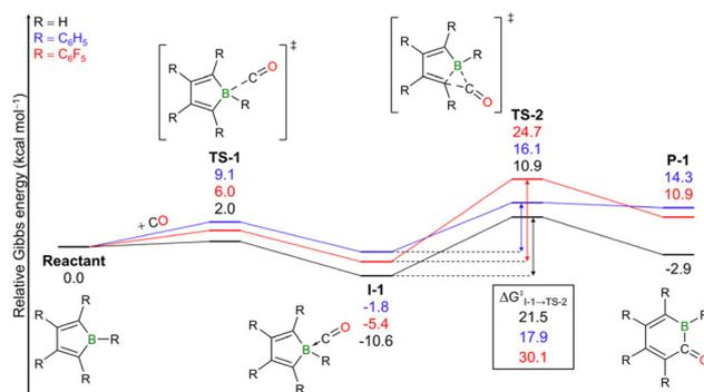
**Fig. 1** Relative Gibbs energy profiles (kcal mol<sup>–1</sup>) in the gas phase for the ring expansion reaction of selected borole derivatives with CO.
