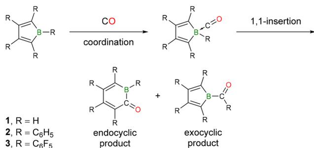
**Scheme 1** A plausible reaction mechanism for the CO insertion into boroles (R = –H, –C<sub>6</sub>H<sub>5</sub>, –C<sub>6</sub>F<sub>5</sub>). The endocyclic product refers to the ring expansion reaction.
