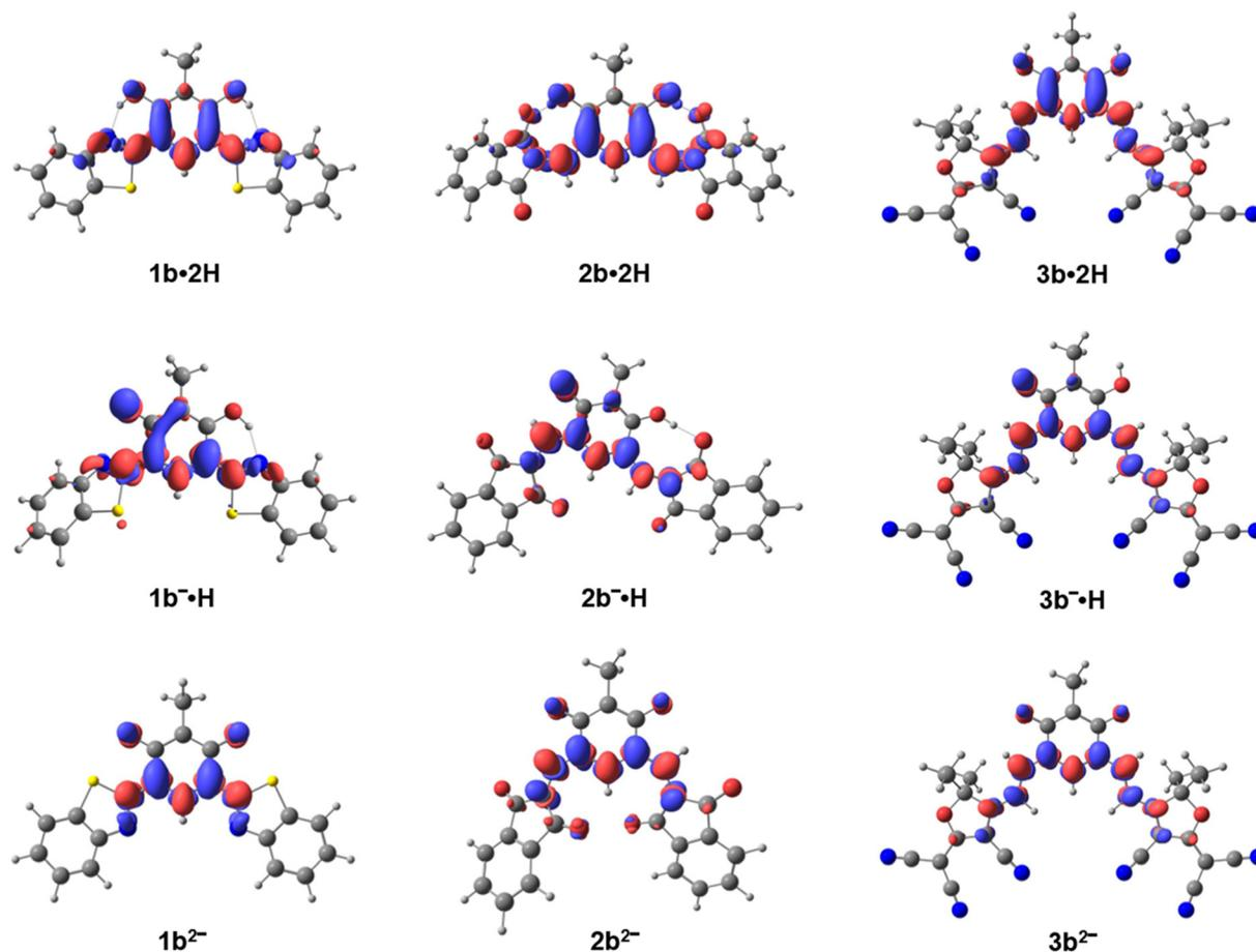
**Fig. 5** Electronic density differences (EDD) between the ground ( $S_0$ ) and the first excited state ( $S_1$ ) for molecules **1b**, **2b** and **3b** (most stable isomers) under different protonation states. Regions in red indicate an increase in electronic density from  $S_0$  to  $S_1$ , while regions in blue indicate a decrease. The isosurfaces are visualized with an isovalue of 0.003.
