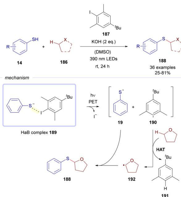
**Scheme 26** Xia's approach to the C(sp<sup>3</sup>)-H bond functionalization reactions for the preparation of thioethers **188**.
