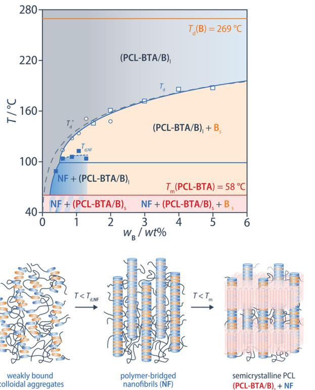
**Fig. 8** Phase diagram of PCL-BTA/B blends constructed from  $T_d^*$  (open circles),  $T_{d,NF}$  (filled squares) and  $T_d$  (open squares) obtained from DSC heating scans of PCL-BTA/B blends.  $(\text{PCL-BTA/B})_l$  – homogeneous melt; NF – nanofibrils;  $B_s$  – bulk B precipitates;  $(\text{PCL-BTA/B})_s$  – solid solution. The grey dashed line indicates fitting of the Flory–Huggins model to  $T_d$  for PCL/B (see Fig. 2).
