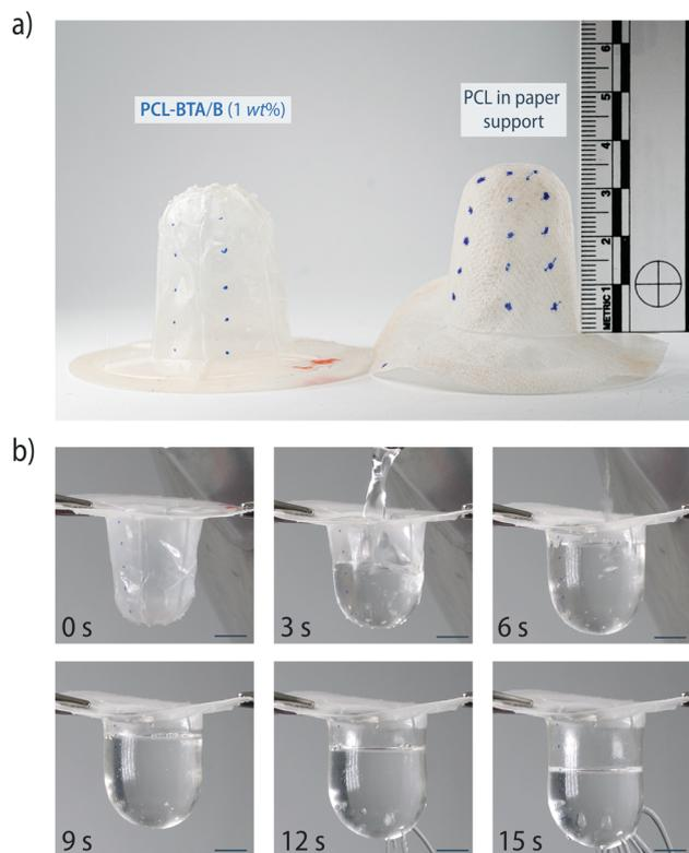
**Fig. 10** (a) PCL-BTA/B (1 wt%) has been processed into cup-shaped objects by thermoforming, whereas pristine PCL can only be thermoformed with the aid of a paper support. (b) The PCL-BTA/B cups were filled with boiling water. Defects associated with the connection of the mold to the vacuum pump during thermoforming resulted in water leakage after 12 s but the cups remained globally intact. Scale bars represent 1 cm.
