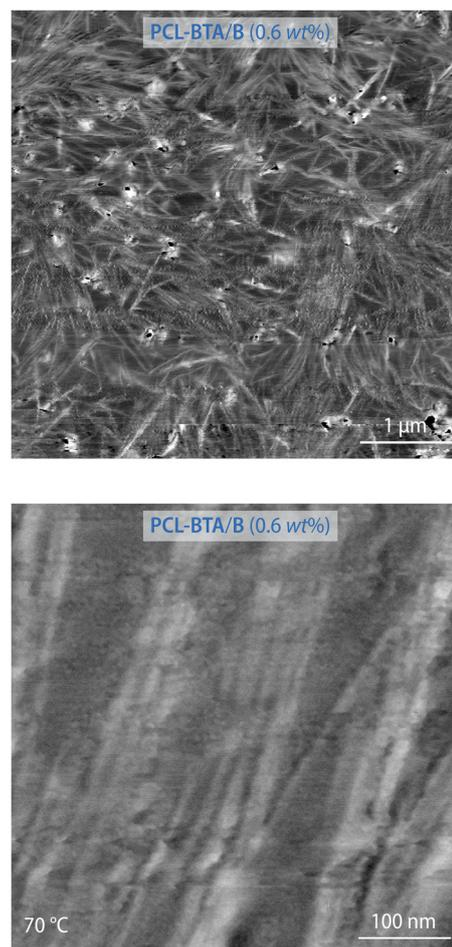
**Fig. 6** Intermittent-contact AFM phase images of PCL-BTA/B (0.6 wt%) recorded at  $70\text{ }^{\circ}\text{C}$  at different magnifications. See ESI Fig. S13.<sup>†</sup>
