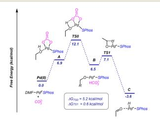
Fig. 7 DFT-calculated reaction profile and solution-state Gibbs free energies ( $\Delta$ GDMF, kcal mol<sup>-1</sup>) at the B3LYP/DEF2-TZVP level of theory at 298 K for stationary points of mechanism A.
