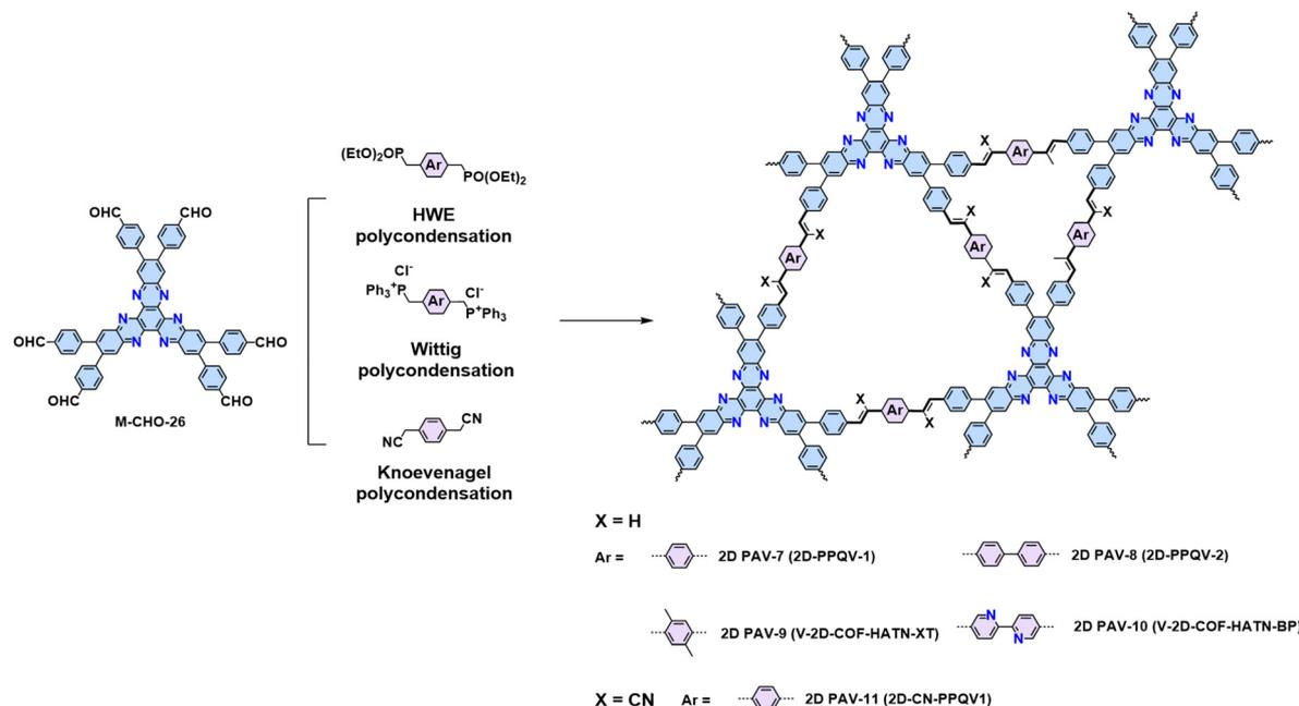
**Scheme 9** Synthesis of 2D PAV-7 (2D-PPQV-1), 2D PAV-8 (2D-PPQV-2), 2D PAV-9 (V-2D-COF-HATN-XT), and 2D PAV-10 (V-2D-COF-HATN-BP) through HWE or Wittig polymerization, together with 2D PAV-11 synthesized by Knoevenagel polycondensation.
