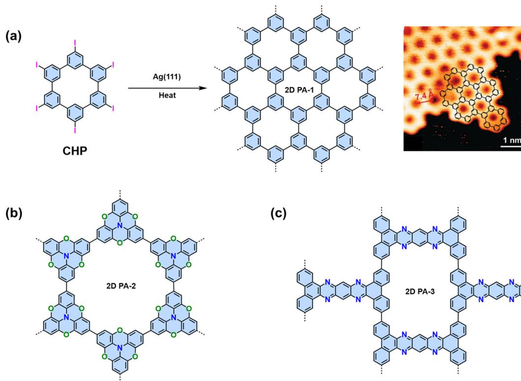
**Fig. 7** (a) On-surface synthesis of 2D polyphenylene (2D PA-1) and the corresponding STM image. (b) Chemical structure of 2D PA-2 synthesized on Au(111) surface. (c) Chemical structure of 2D PA-3 synthesized by solid-state synthesis.
