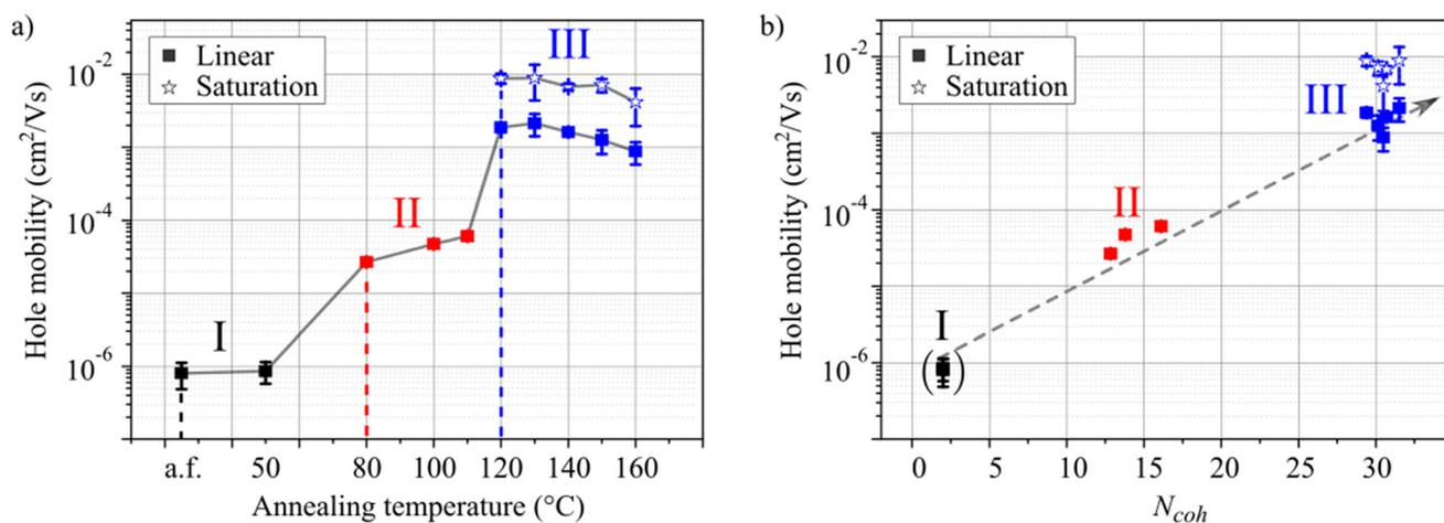
**Fig. 5** Hole mobility as a function of molecular aggregation. (a) Experimental hole mobilities of HB238 thin films spin-coated on OFET substrates for a non-annealed sample [as fabricated (a.f.)] and for samples after annealing at different temperatures between 50 °C and 160 °C for 10 minutes each. (b) Hole-mobilities as a function of the estimated number of coherently coupled molecules extracted from the absorbance spectra in Fig. 2a. The dashed grey arrow is a guide to the eye.
