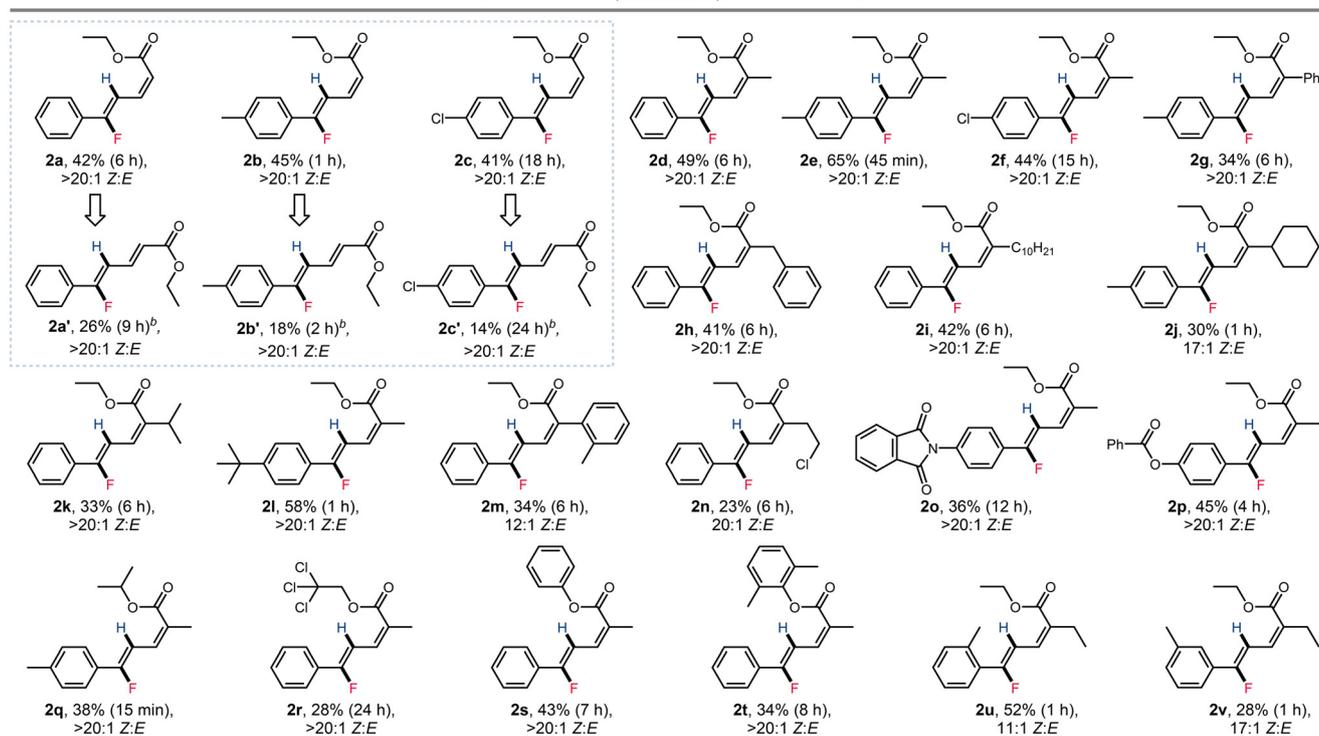
**Scheme 2** Substrate scope for the formation of fluorinated dienoates **2**. <sup>a</sup> Reaction conditions: **1** (0.25 mmol), 2,6-dichloropyridinium tetrafluoroborate (0.50 mmol), chloroform (5.0 mL), stirred at 70 °C for indicated duration. <sup>b</sup> 1,2-DCE (0.05 M) was used as solvent.
