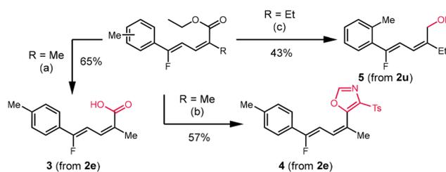
**Scheme 3** Divergent transformations of products. (a) LiOH (4.0 equiv.), THF (0.5 M), 50 °C, 24 h. (b) TosMIC (1.0 equiv.), *n*BuLi (2.0 equiv.), THF (0.5 M), 0 °C, 4 h. (c) DIBAL-H (3.0 equiv.), THF (0.5 M), 0 °C, 2 h.
