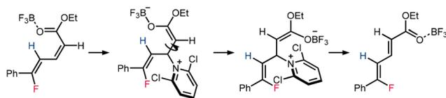
Scheme 5 Proposed mechanism for isomerization of dienoate **2a**.
