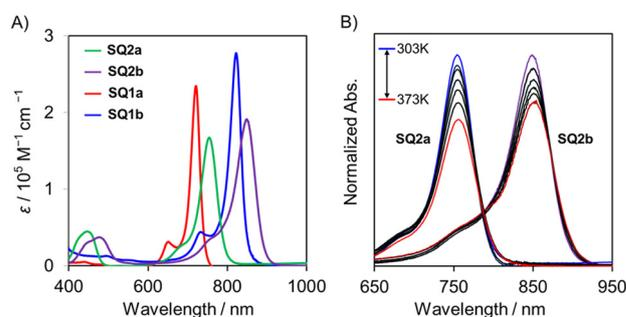
**Fig. 6** (A) The electronic absorption spectra of **SQ2a** (green), **SQ2b** (purple), **SQ1a** (red) and **SQ1b** (blue) in DMSO (5  $\mu$ M). (B) Normalized electronic absorption spectra of **SQ2a** and **SQ2b** in the temperature range from 373 to 303 K.
